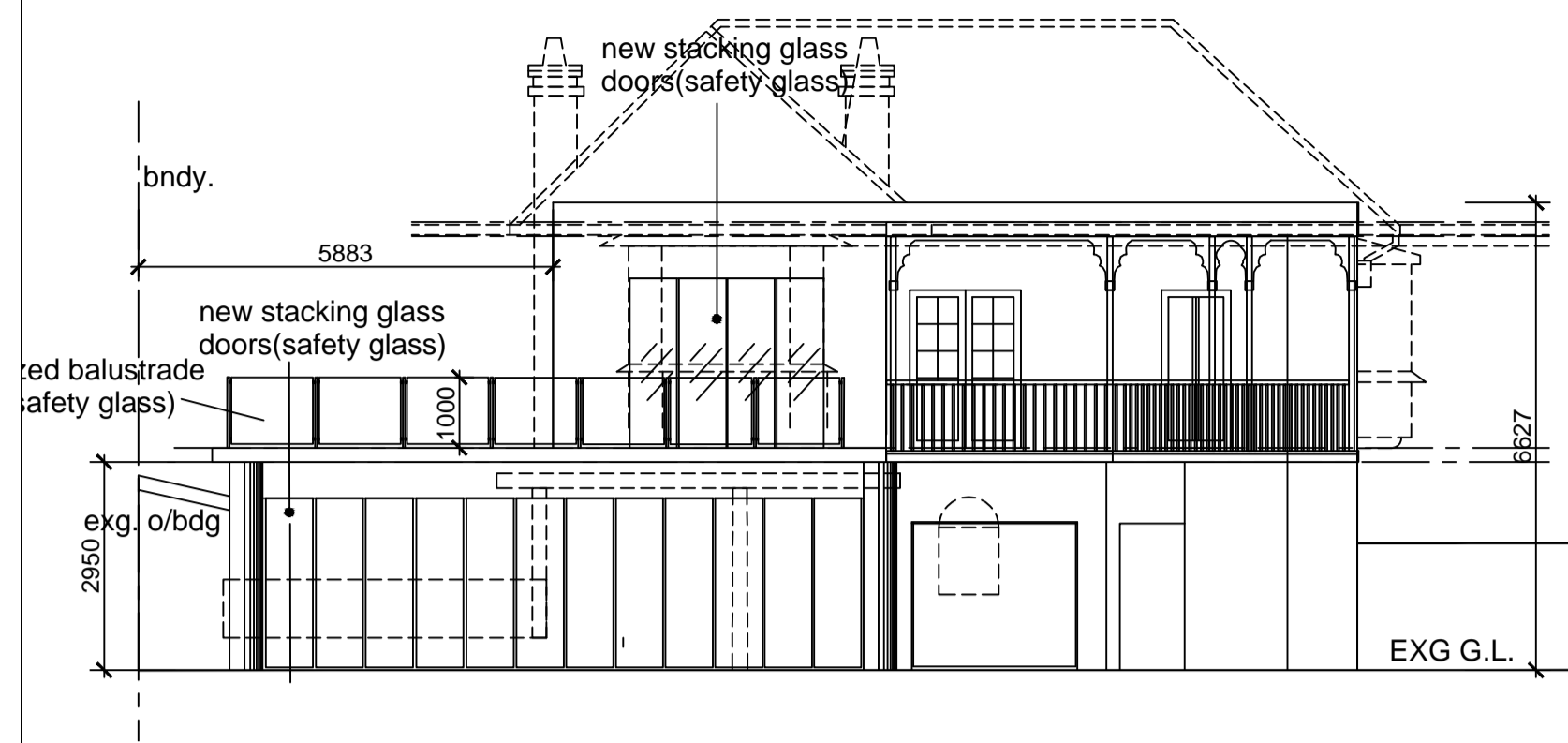
NORTH EAST ELEVATION SCALE 1:100
