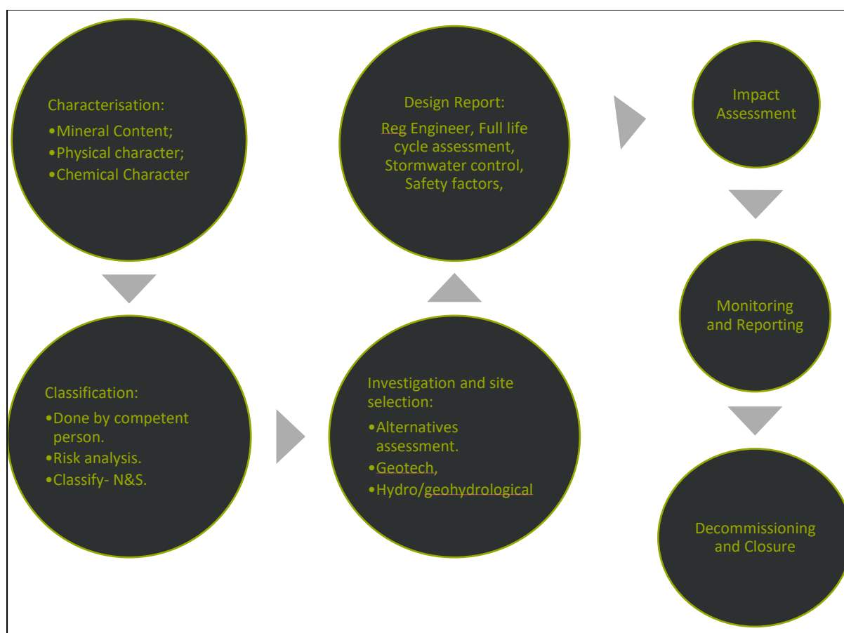
Figure 17: Overview of the planning and management of residue stockpiles and residue deposits regulations.
