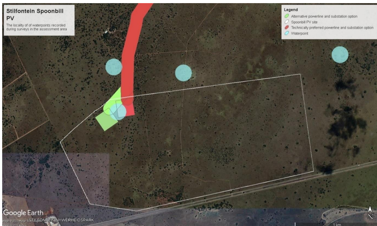
Figure D1: Spoonbill PV sensitivities map showing waterpoints, powerline options and on-site substation options.
