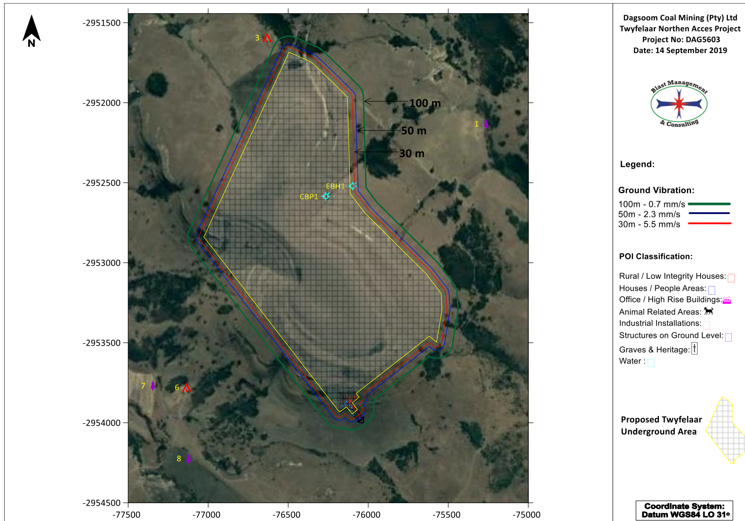
Figure 20: Ground vibration influence from underground blasting operations
