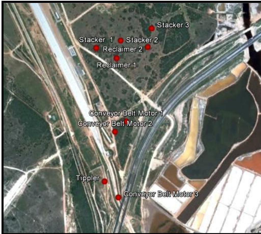
Figure 12-1: Location of noise generating equipment at the proposed Mn ore terminal
