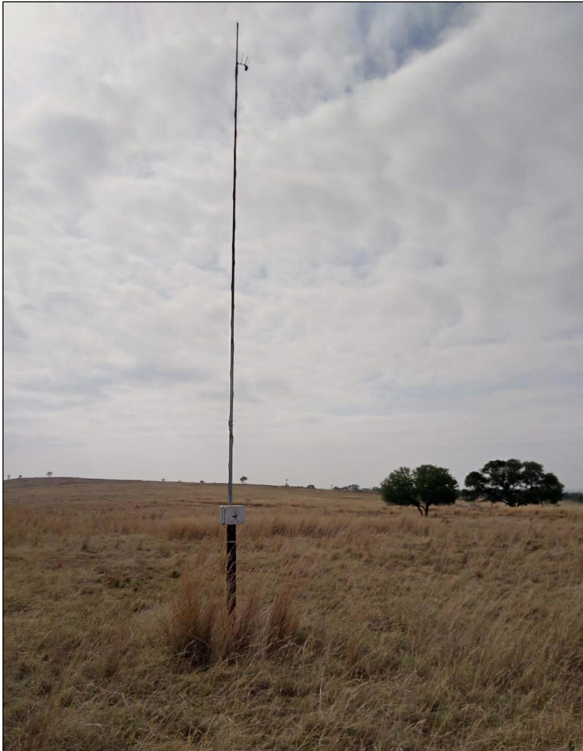
Figure 3-1. The passive bat detection system on Short Mast 1 (ShM1)
