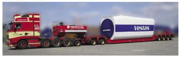
Figure 4-1:Transporting the Nacelle (Dvorak, 2010)
