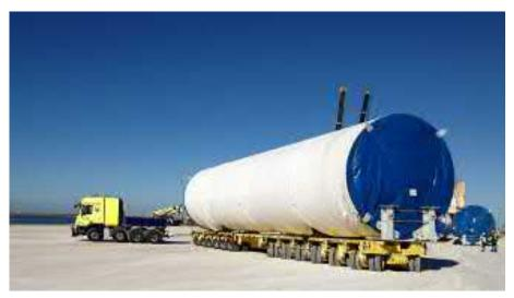
Figure 4-3:Transporting the Tower Sections (Montiea, 2014)
