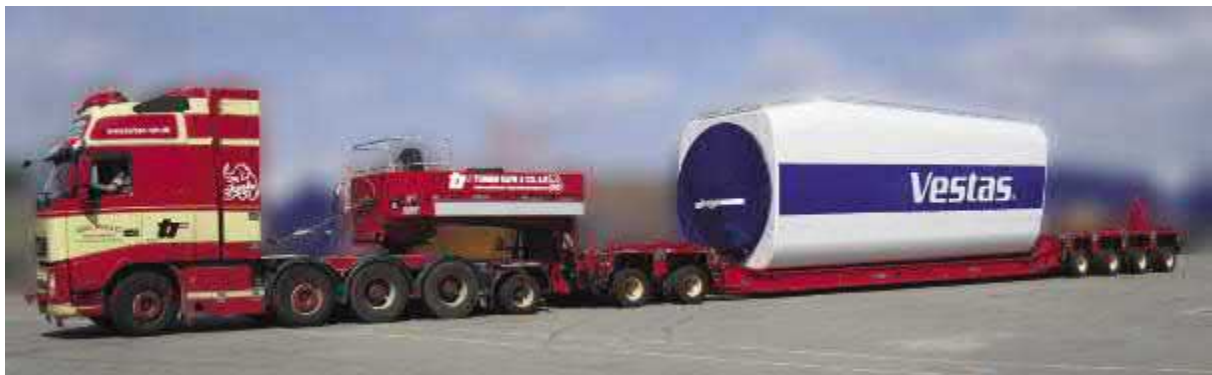
Figure 4-1:Transporting the Nacelle (Dvorak, 2010)
