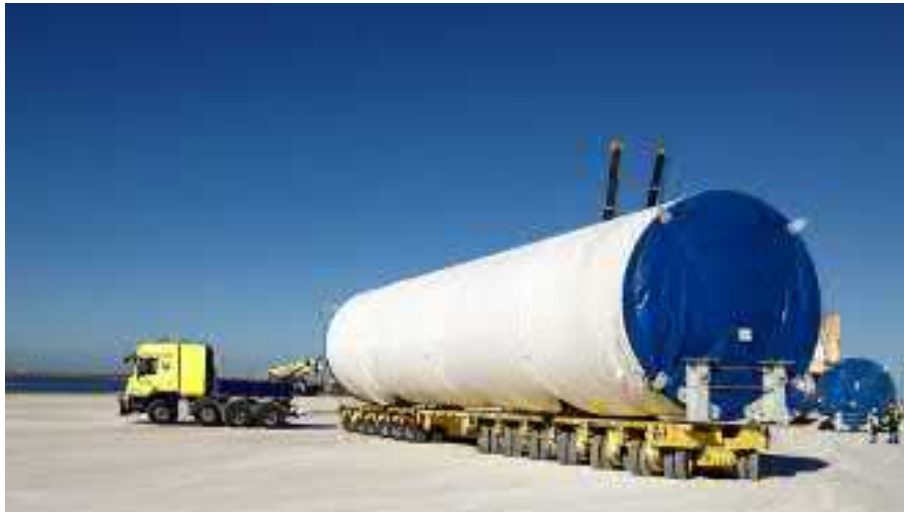
Figure 4-3:Transporting the Tower Sections (Montiea, 2014)
