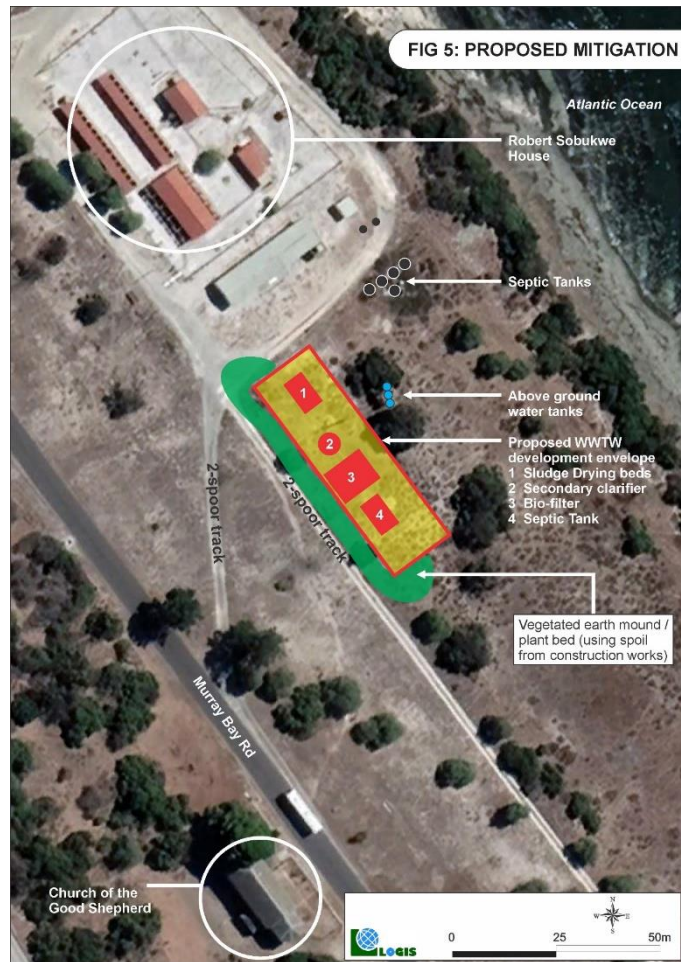
Figure 7-1: Location of vegetated earth mound
