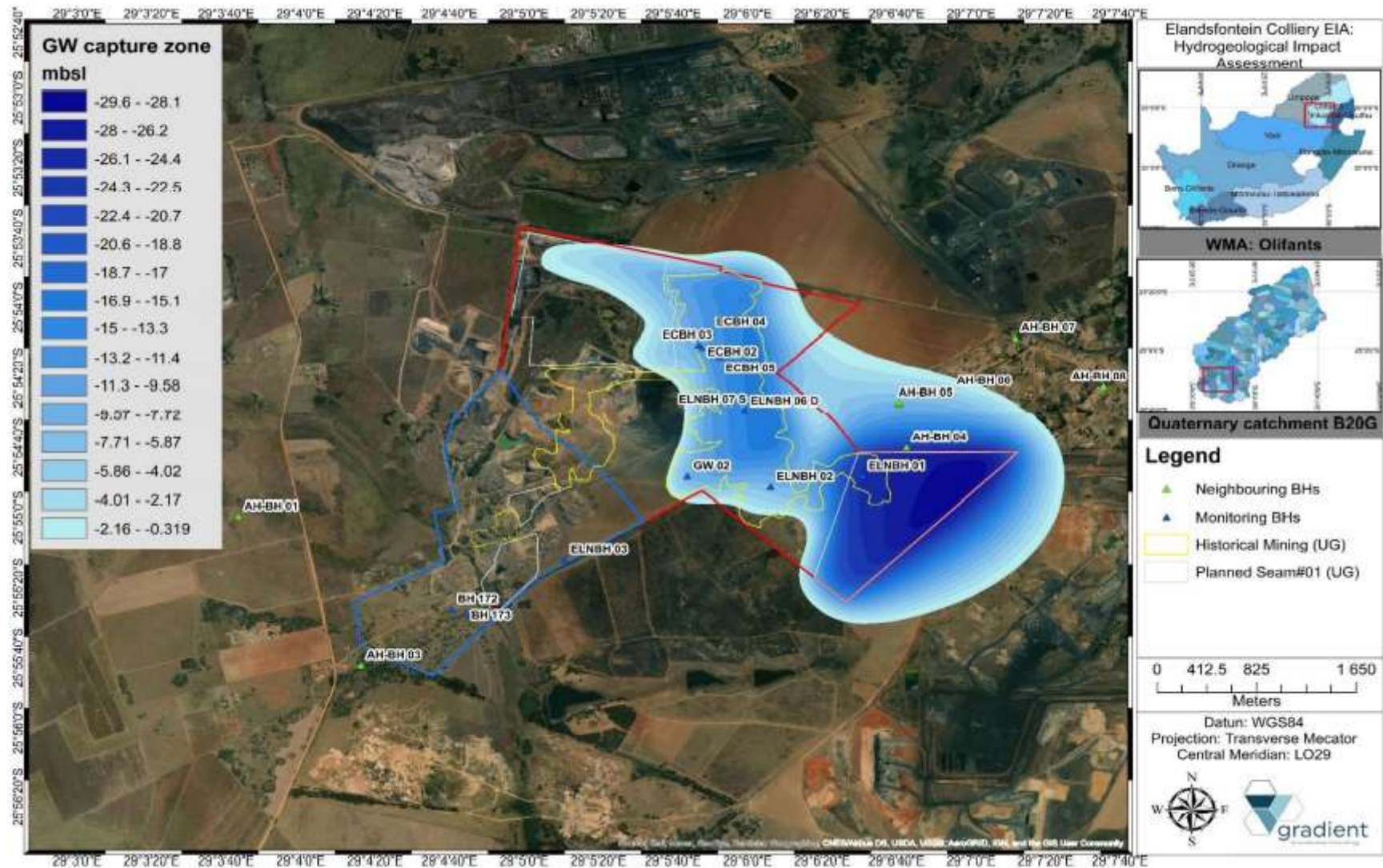
Figure 33: Water level drawdown and groundwater capture zone of the deeper, fractured aquifer.
