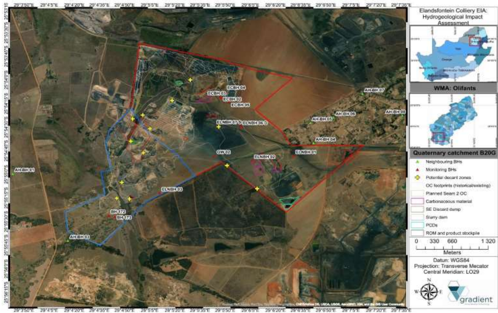
Figure 37: Potential high-risk decant zone for the backfilled opencast pits
