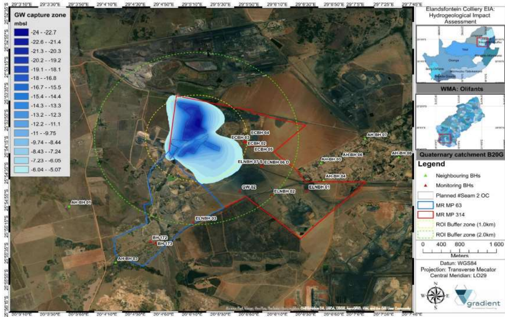
Figure 32: Water level drawdown and groundwater capture zone of the shallow, weathered aquifer.
