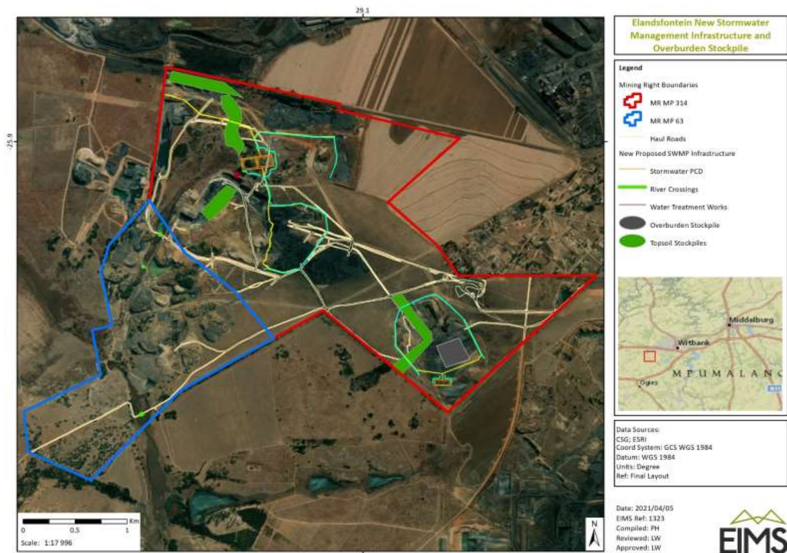
Figure 24: Updated Layout Map indicating new stormwater management infrastructure proposed as part of the Elandsfontein EA application as well as location of new overburden stockpile and topsoil stockpiles.
