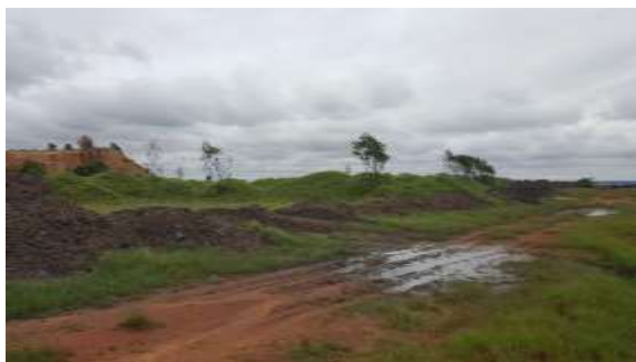
Figure 4: Topsoil (foreground) and softs (background) stockpiles, eastern side of ptn 7.
