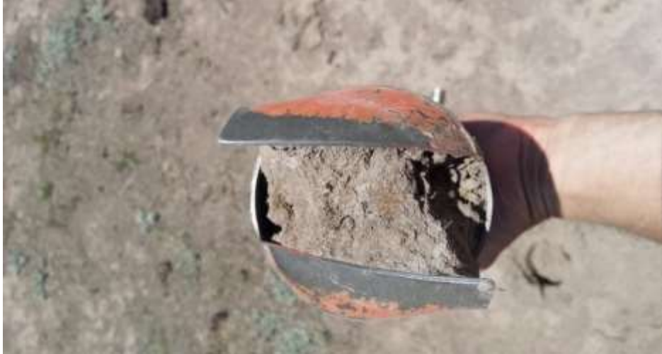
Figure 33: Iron Concentrations and Depleted Soils within the Pan Wetlands with the Soft Plinthic Soil Horizon
