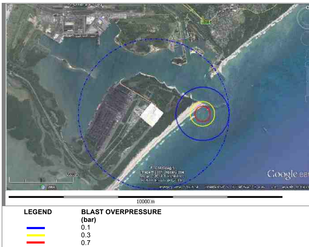
Figure 20: Blast overpressures for the worst-case vapour cloud explosion from a release from a single 7882 m 3 LPG storage vessel
