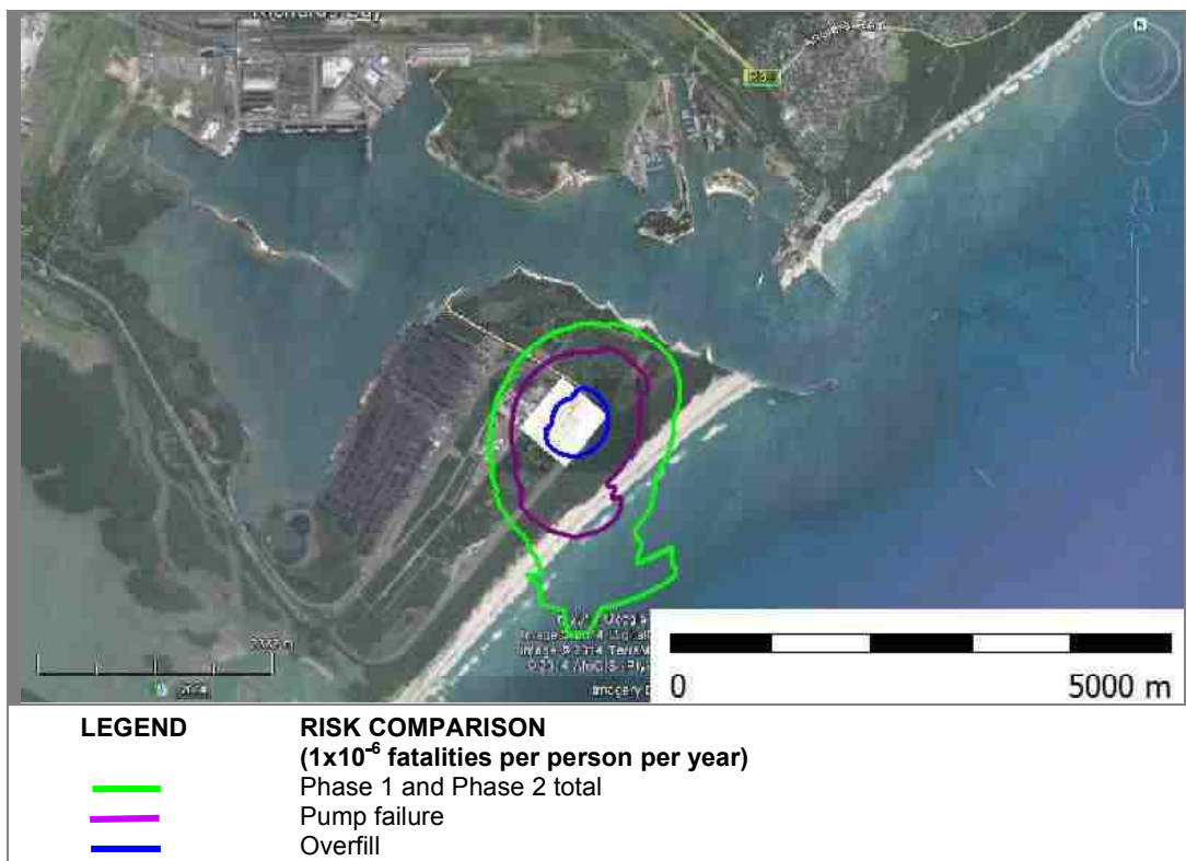
Figure 24: Comparison of the risk of 1 \times 10^{-6} fatalities per person per year isopleths
