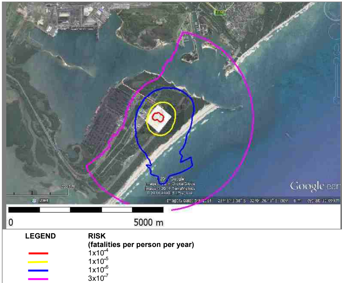
Figure 23: Risk contours for LPG releases at the bulk storage and gantries
