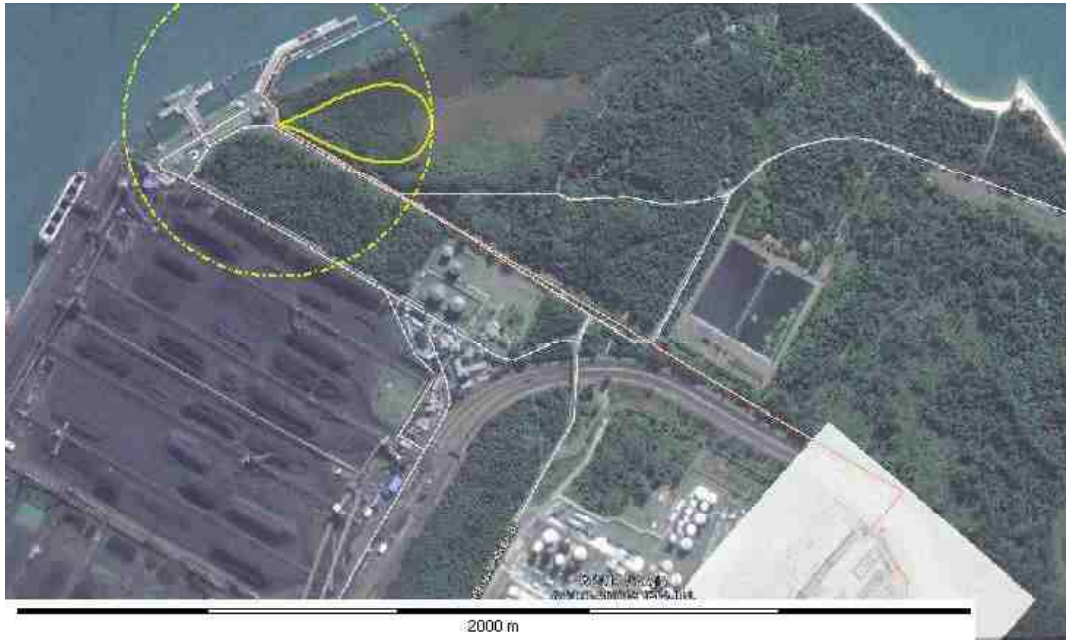
Figure 49: The Extent of a Flash Fire from a LPG Pipeline Failure as Indicated by the LFL.
