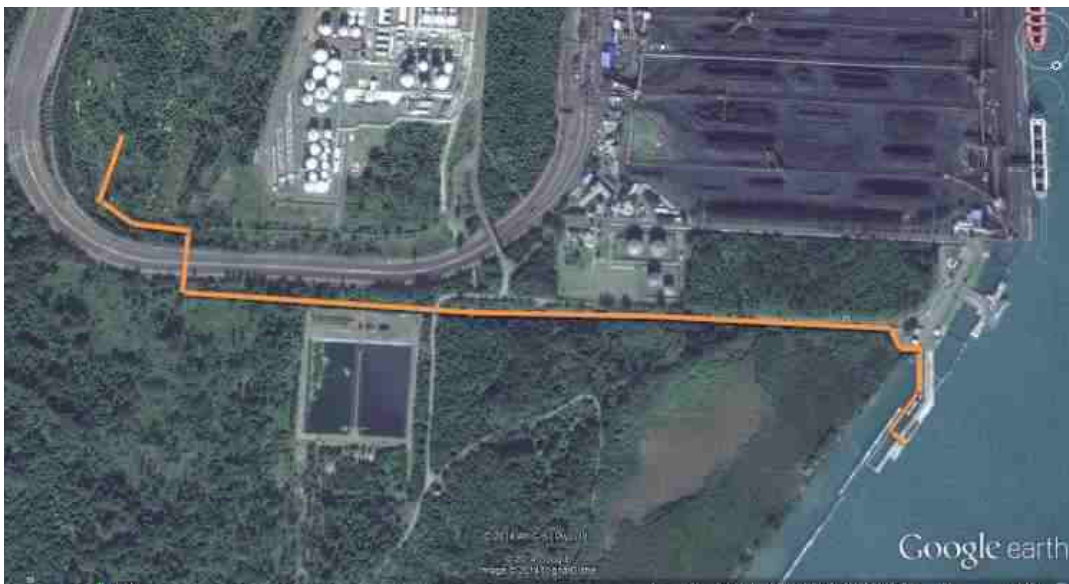
Figure 6: Proposed routing of the pipelines from the berths to the tank farm
