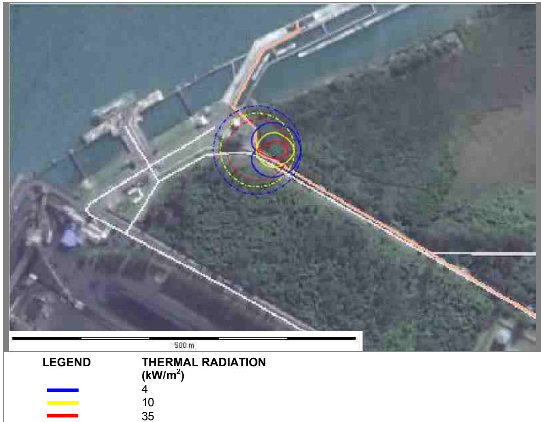
Figure 11: Thermal radiation for a jet fire from a release from a 25 mm hole in the LPG pipeline
