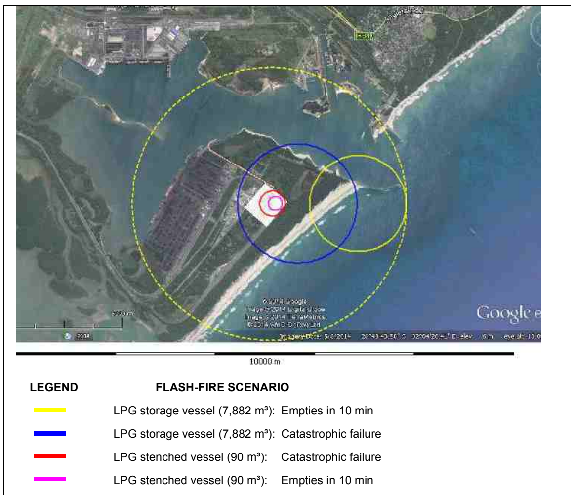
Figure 56: Maximum Distances to the 0.1 Bar Overpressure for LPG VCEs at the Initial Phase Storage.
