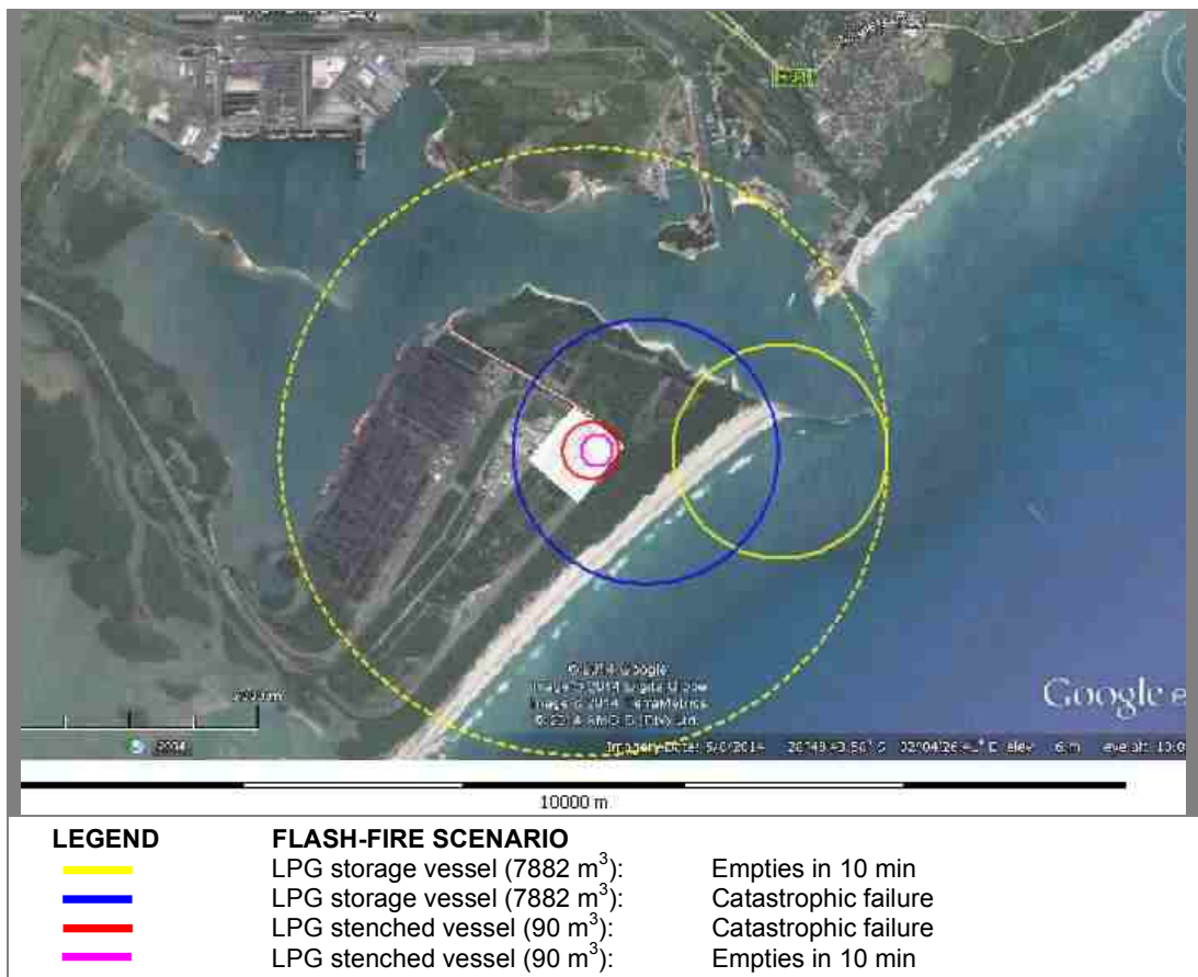
Figure 19: Maximum distances to the 0.1 bar overpressure for LPG VCEs at Phase 1 storage
