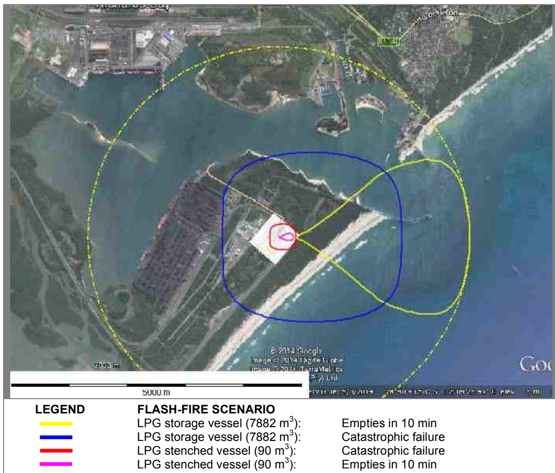
Figure 18: Maximum extent of the impact from LPG flash fires at Phase 1 storage
