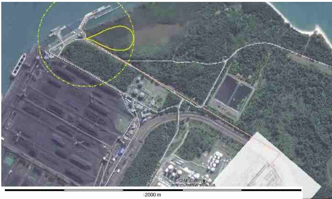
Figure 12: The extent of a flash fire from a LPG pipeline failure as indicated by the LFL
