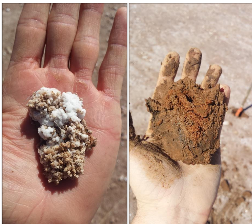
Figure 60: Salt Precipitation at the Surface (left) and Red Iron and Black Manganese Accumulations observed in the Sub-soils of a Saline Wetland
