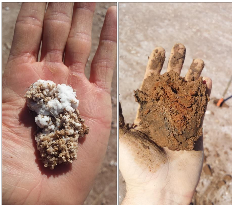
Figure 59: Salt Precipitation at the Surface (left) and Red Iron and Black Manganese Accumulations observed in the Sub-soils of a Saline Wetland
