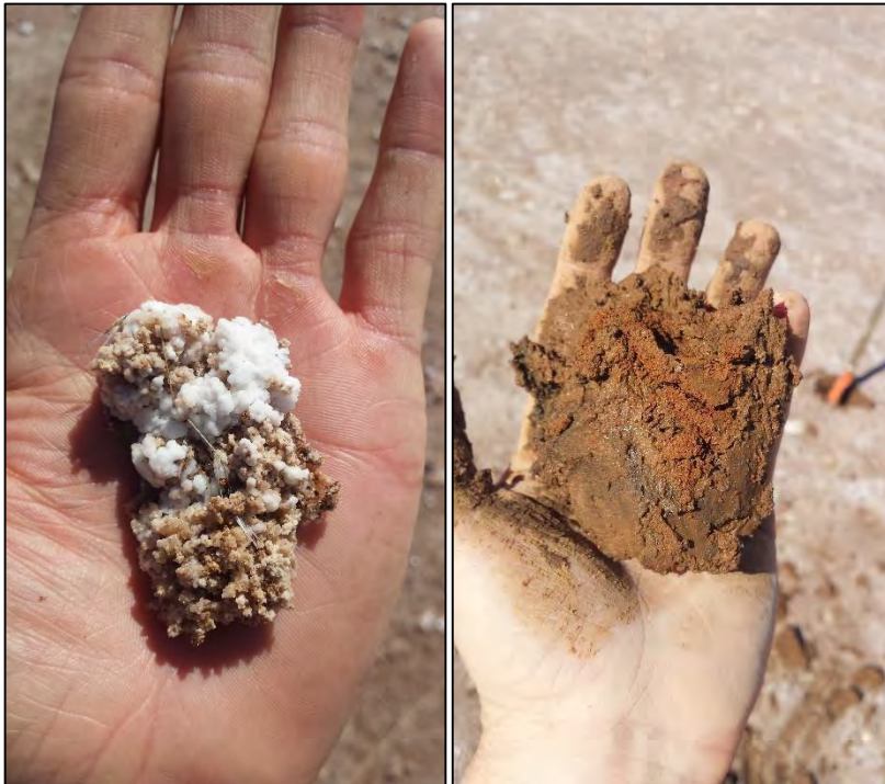
Figure 90: Salt Precipitation at the Surface (left) and Red Iron and Black Manganese Accumulations observed in the Sub-soils of a Saline Wetland
