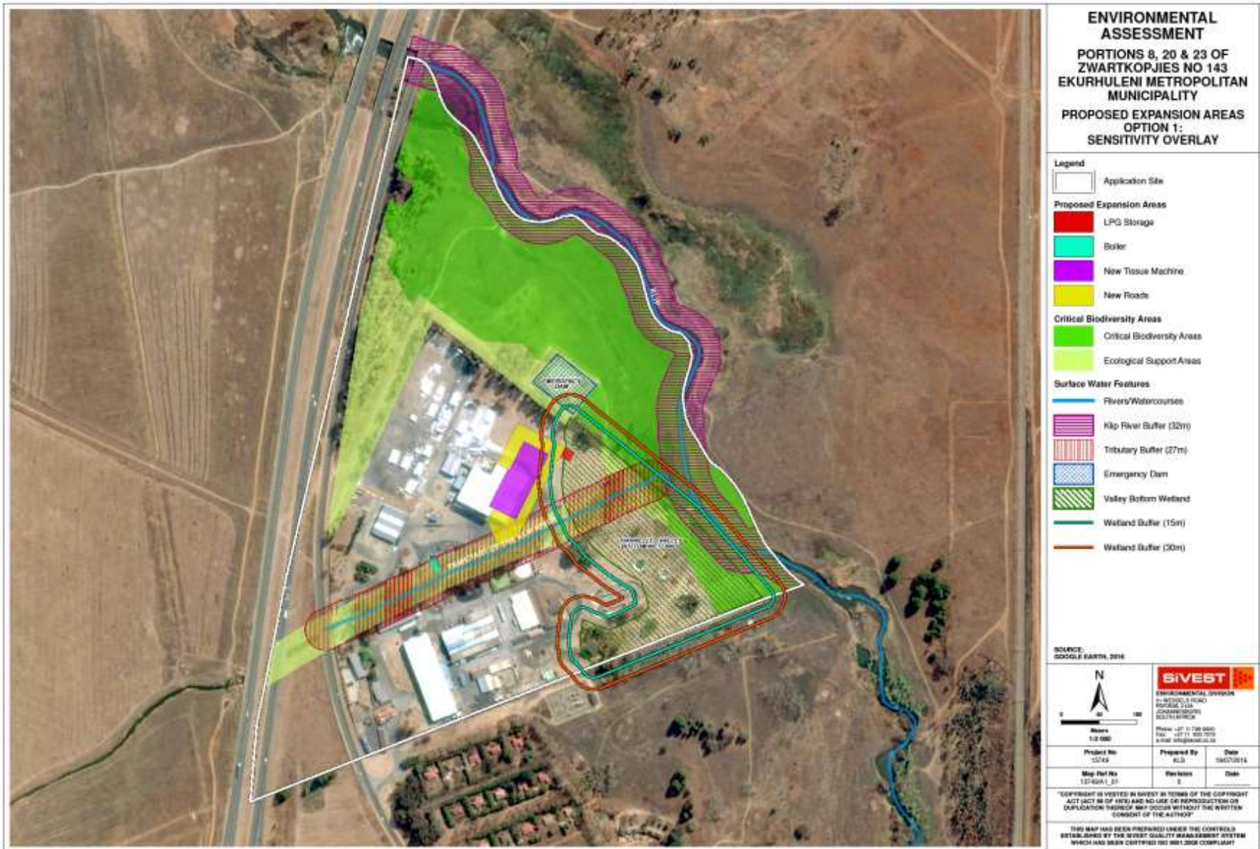
Figure 11: Site Layout Map for Option 1 indicating the sensitive areas identified within the existing Twinsaver Kliprivier Paper Mill site
