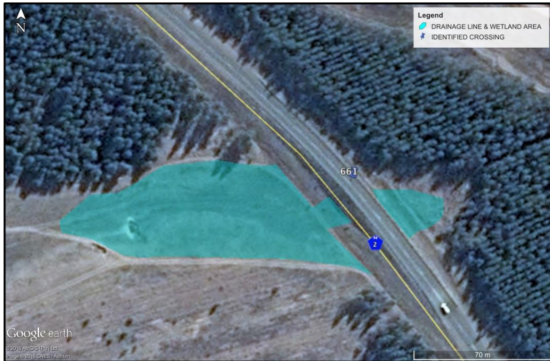
Figure 18: 661 – Drainage line and associated wetland (seep) area
