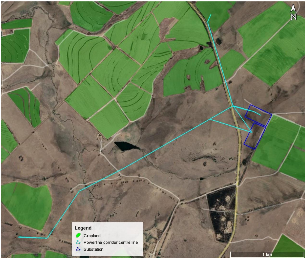
Figure 3. Satellite image map of all proposed alternative powerline routes (light blue lines) and alternative substation sites (dark blue outlines). Note that a 500m wide powerline corridor (250m either side of the centre lines) is the subject of this assessment.
