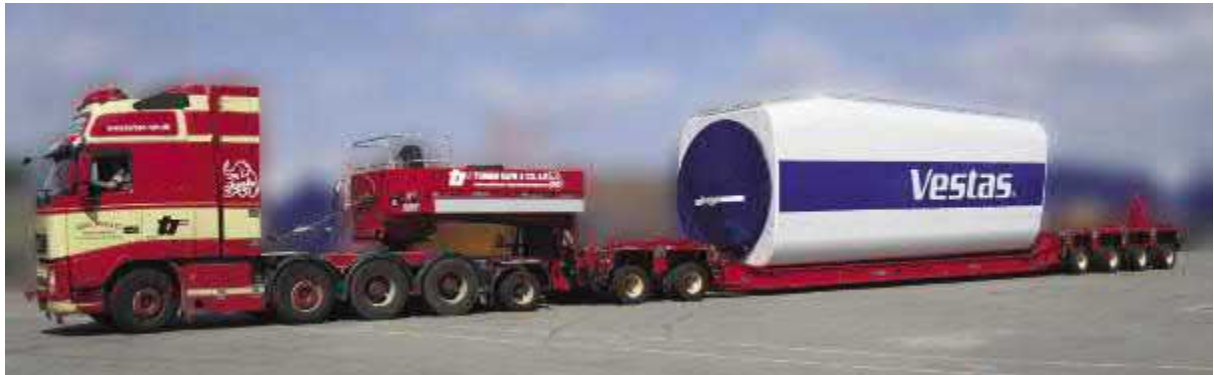
Figure 4-1: Transporting the Nacelle (Dvorak, 2010)
