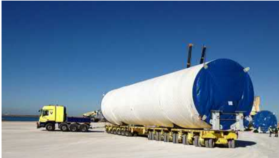
Figure 4-3: Transporting the Tower Sections (Montiea, 2014)
