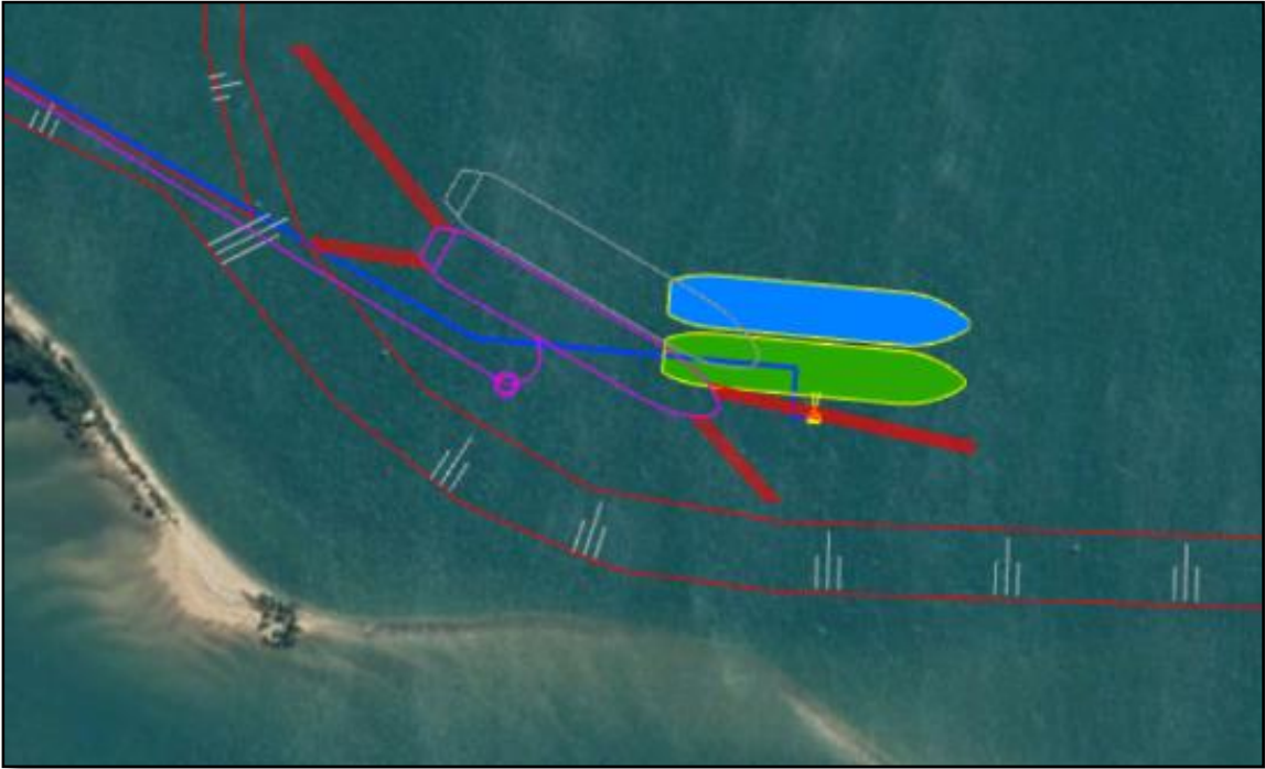
Figure 7-2: Deviation of the FSRU and LNGC positions
