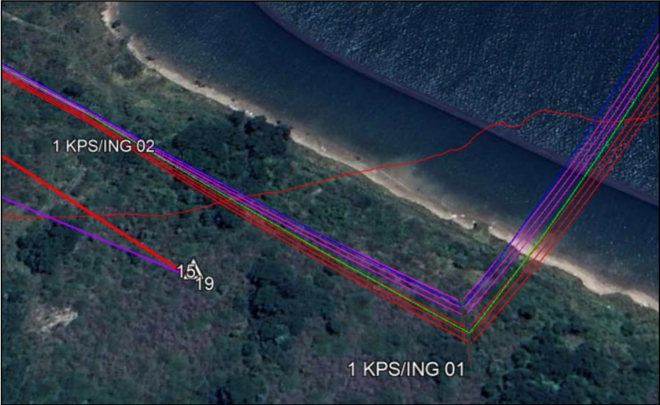
Figure 7-1: Transmission line – deviation of the start point.
