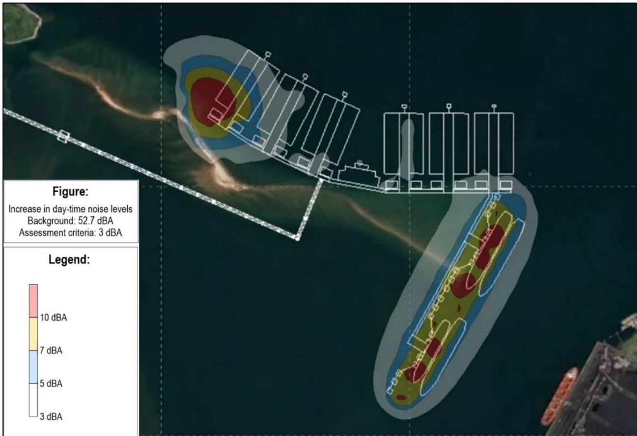
Figure 116: Simulated increase in equivalent continuous day-time rating level ( \Delta L_{Req,d} ) above the baseline (i.e. 52.7 dBA)
