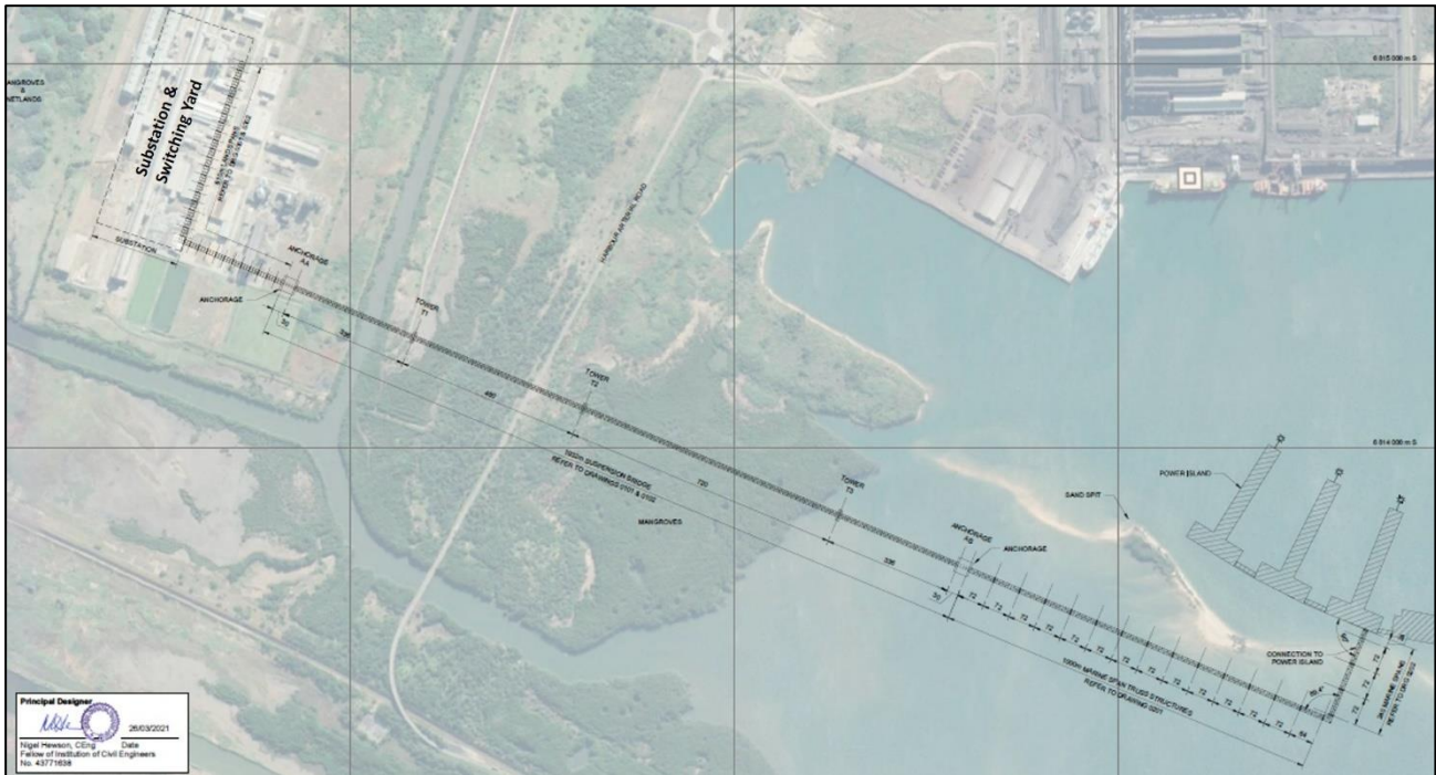
Figure 16: Route alignment and location of main anchorage chambers/ platforms and towers for the pipe and cabling bridge structure to evacuate power from the NIFPP to the land-based substation.
