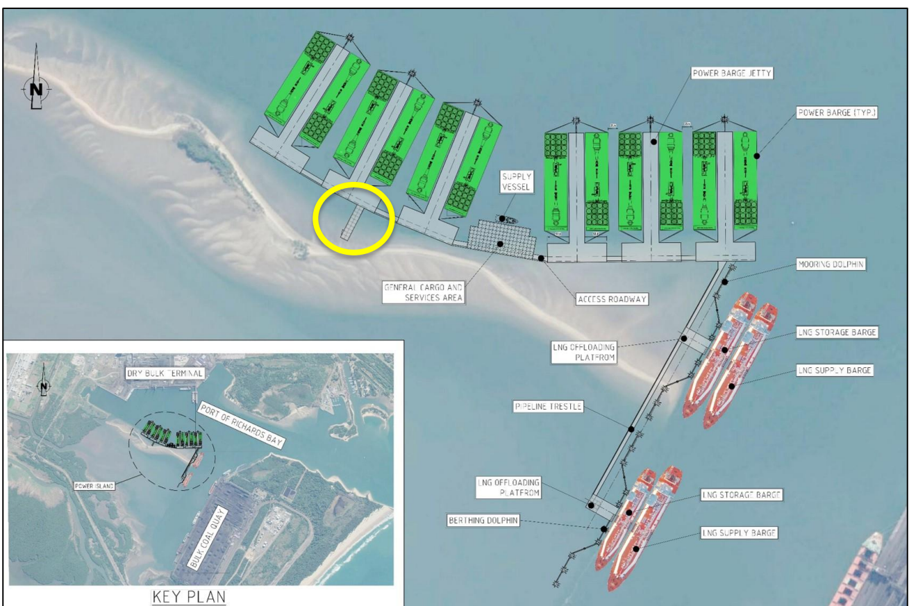
Figure 110: Revised Layout with the transformer platform shifted more to the east (highlighted by the yellow circle) along the Power Barge Terminal to avoid the sandspit Mangrove Forest patch (as per specialist recommendation).
