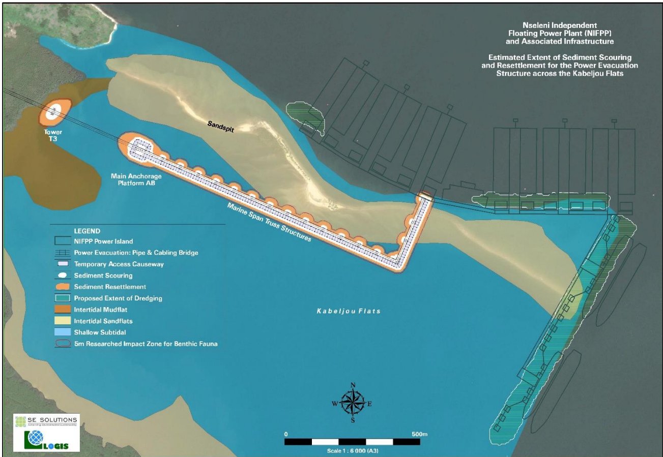
Figure 114: Scour (white) hole and resettlement of sediment (deposition – orange) and 5m impact zone associated with the initial impact of the construction of the Pipe and Cabling Bridge (including temporary works) within the Kabeljous Flats.
