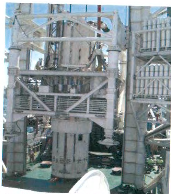
Figure 2: The 2.5 m diameter drill bit within the drill frame structure.
