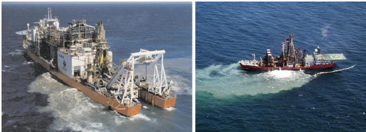
Figure 81: Typical crawler-vessel (left) and drillship (right) operating in the Atlantic 1 Mining Licence Area.
