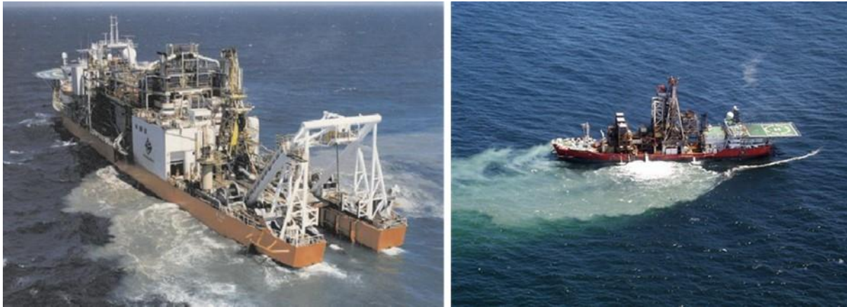
Figure 71: Typical crawler-vessel (left) and drillship (right) operating in the Atlantic 1 Mining Licence Area.
