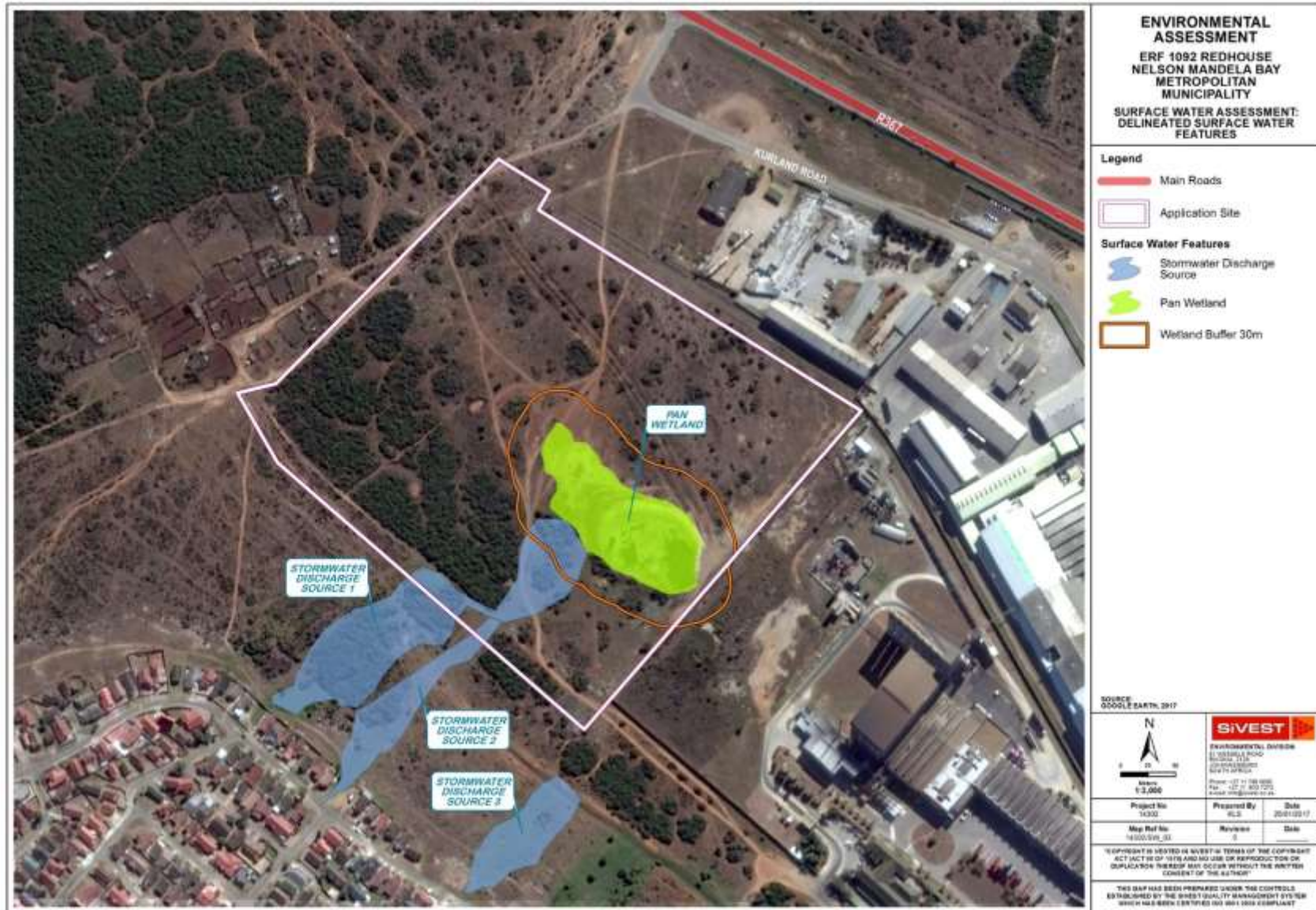
Figure 4: Site locality map indicating the delineated depression wetland found within the proposed project site
