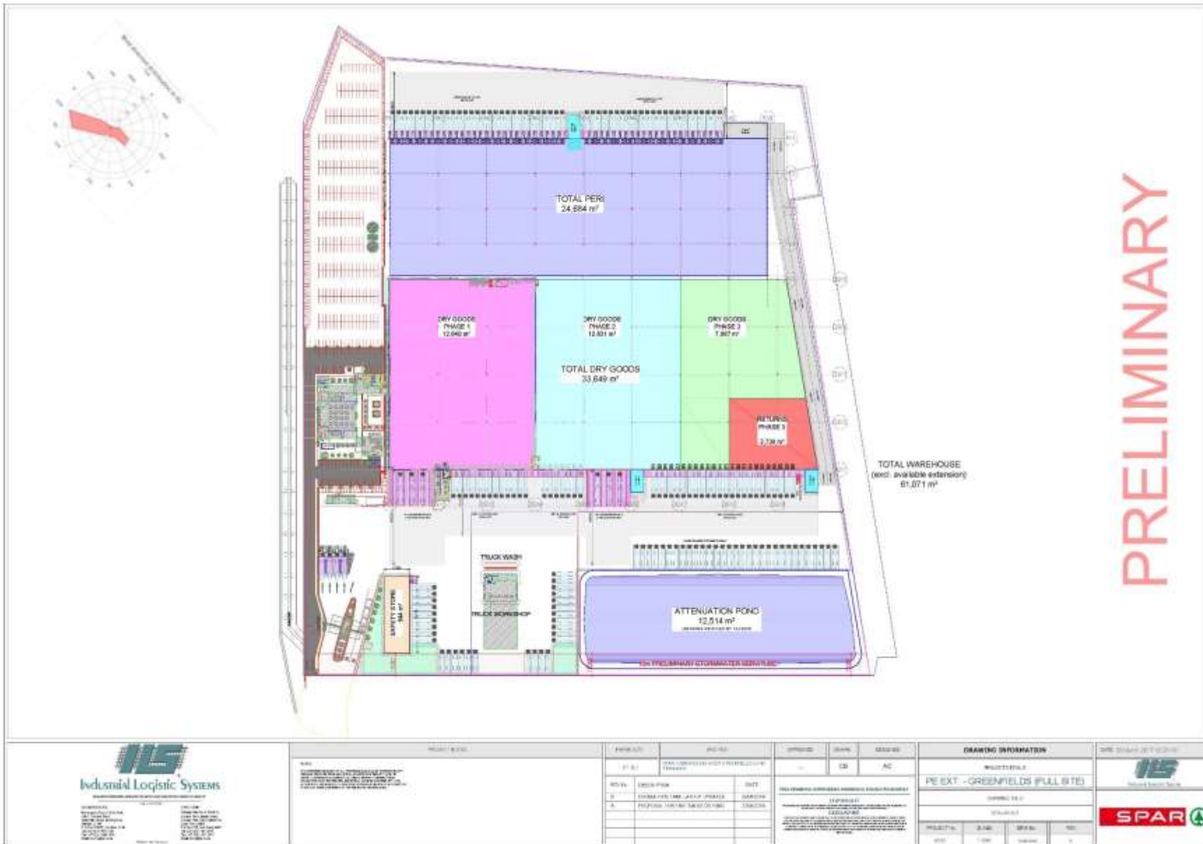
Figure 2: Long term site plan indicating the different components of the proposed development, as well the phasing for each respective component
