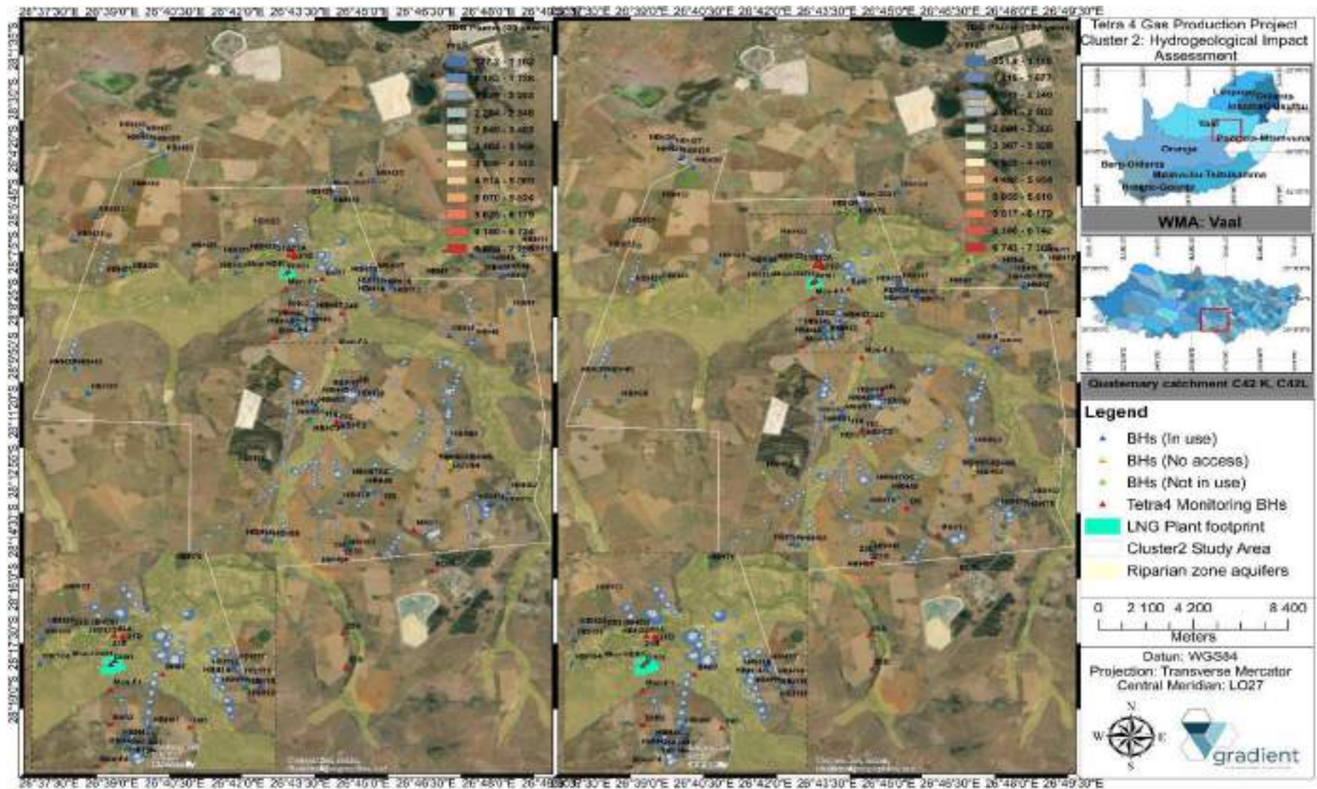
Figure 89: Scenario 04a: TDS pollution plume migration of contaminants originating from the deeper, fractured aquifer migrating through the intergranular aquifer (post-closure phase).
