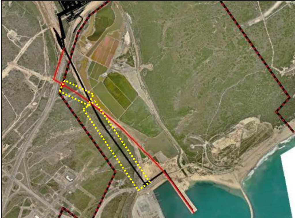
Figure 14B.15: Google earth© satellite image of the IDZ Zone 8 area (Ngqura Port) showing the preferred conveyor belt route (black line) and the alternative route (red line). The preferred route would entail the excavation of cuttings through potentially fossiliferous sediments of the Kirkwood Formation on the south-western side of the Coega Estuary. The alternative route runs largely along an existing alignment that is already disturbed and sealed-in, so bedrock excavations required here are considerably less. Zones of high palaeontological sensitivity along the conveyor routes are indicated by the yellow dotted rectangles.
