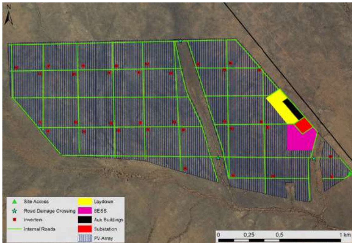
Figure 1. Proposed site layout plan for preferred development option (Dyasonsklip Solar Energy Facility 1)
