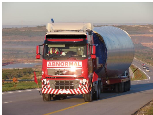
Figure 2-4: Example – Transportation of Tower Sections
