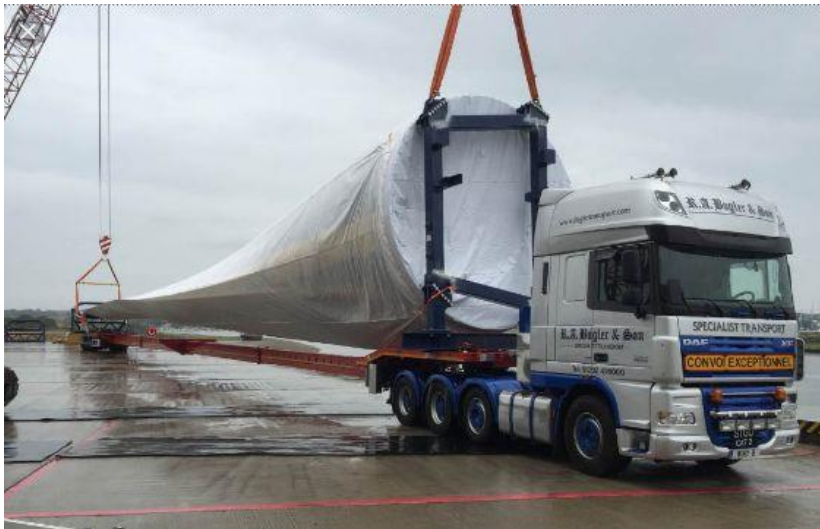
Figure 2-2: Example -Transport of Blades on extendible trailers
