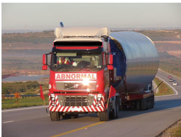
Figure 2-4: Example – Transportation of Tower Sections
