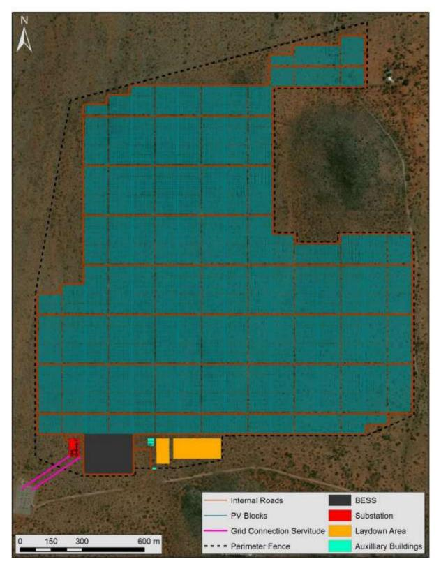
As can be seen above, the proposed BESS is situated in the South West of the approved footprint, adjacent to the on-site substation. The full-sized layout plans are appended to the Amendment Assessment Report and application for amendment form.
