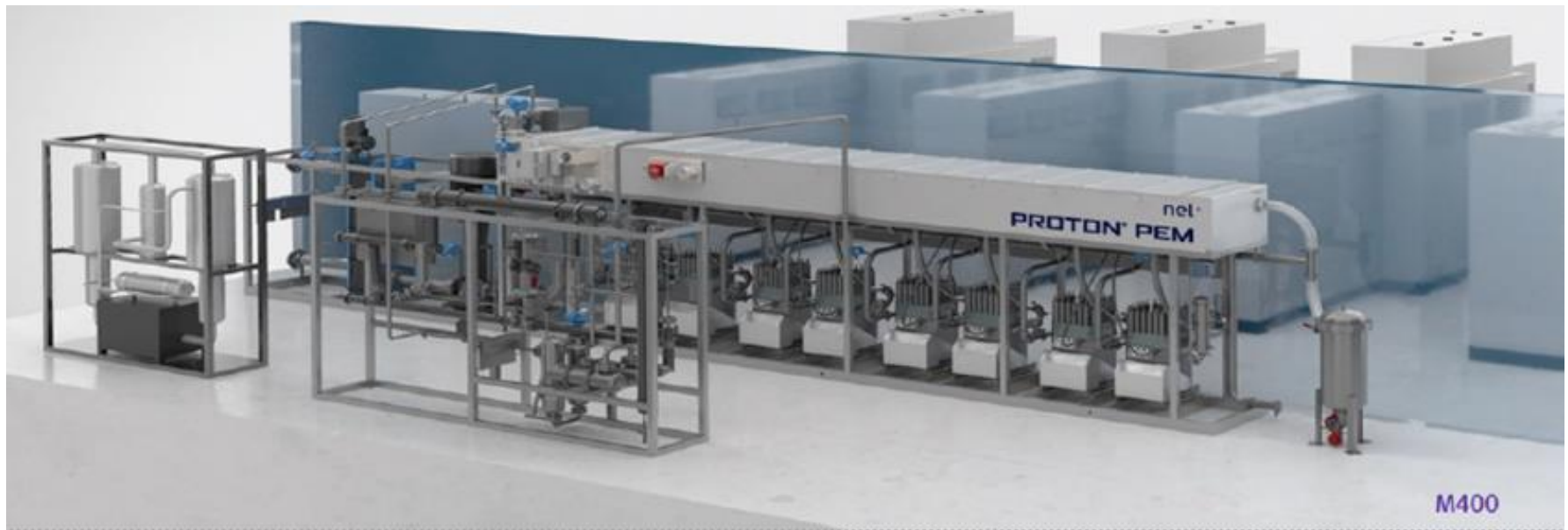
Figure 7: Example of an Electrolyser Unit (Nel Proton PEM)
