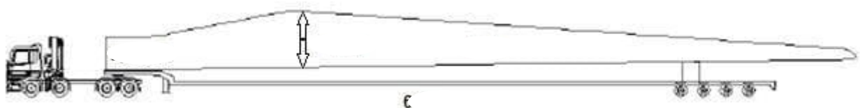
Figure 2-5: Example of Blade Transport
