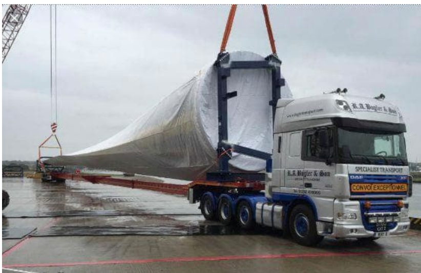
Figure 2-4: Example - Transport of Blades on extendible trailers
