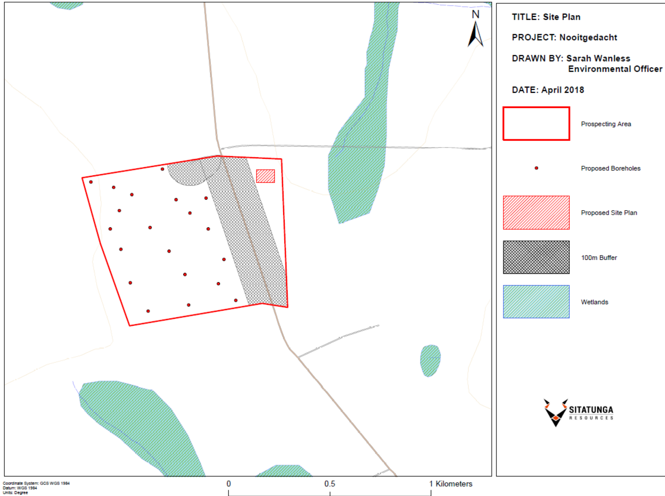
Figure 3 Prospecting Area, Indicating preliminary position of prospecting boreholes in relation to water bodies
