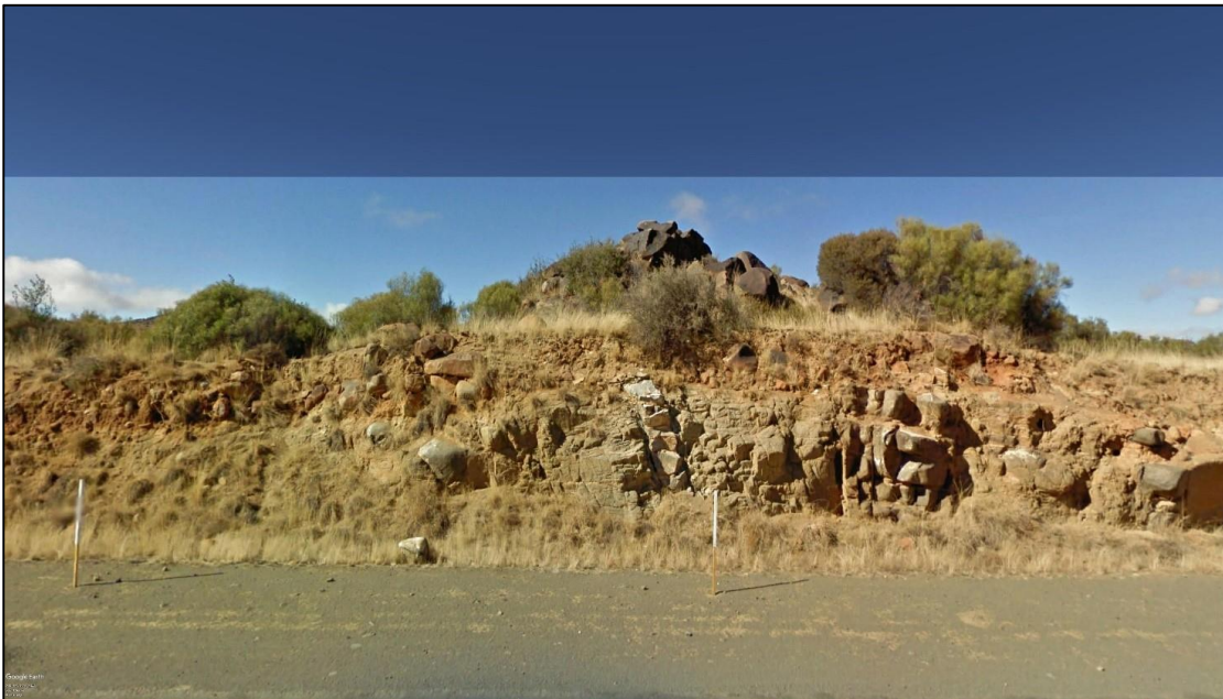
Figure 40: Dolerite weathering profile with corestones and surface boulders (N10 near Mooi Plaats site – Google Earth)
