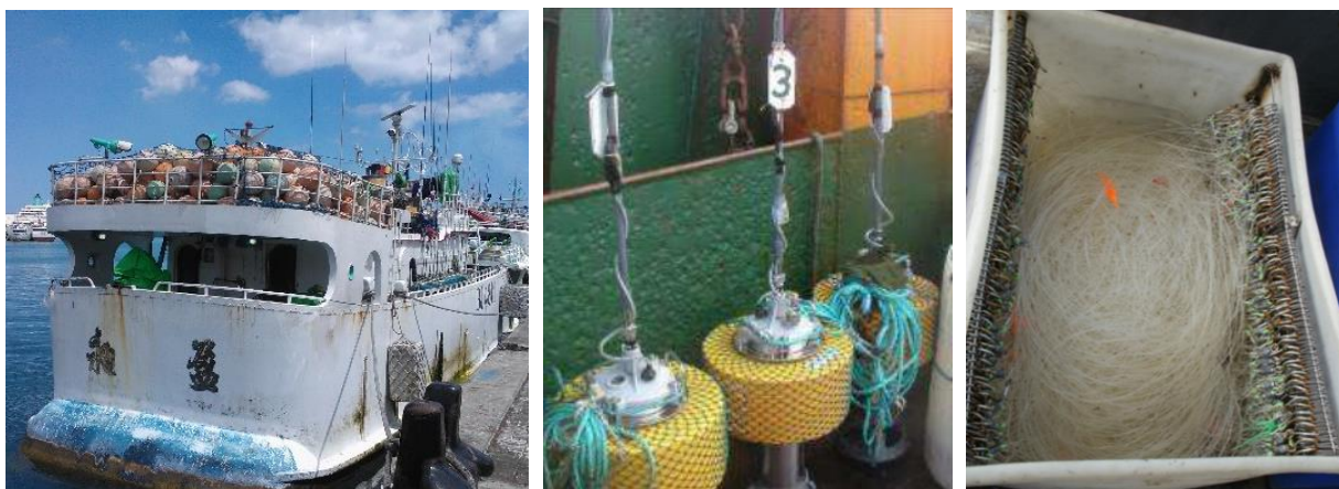
Figure 100: Photographs showing marker buoys (left), radio buoys (centre) and monofilament branch lines (right) (Source: CapMarine, 2015).
