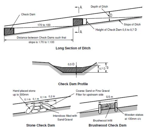
Figure 14:2 Typical Erosion Control
