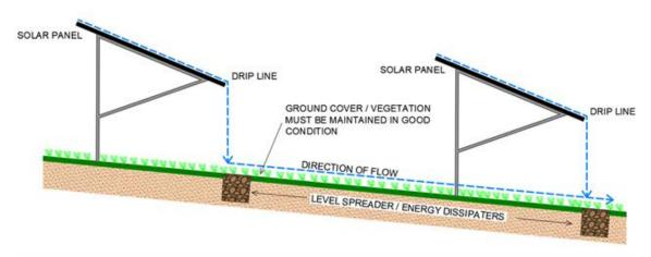
Figure 14:3 Stormwater control of Fixed Tilt PV showing drip line (Conceptual)
