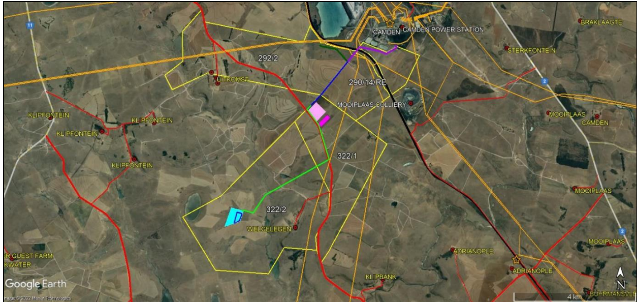
Figure 3.3: Proposed Camden I Green Hydrogen & Ammonia Plant and subject properties (yellow outlines) indicated in relation to existing Eskom lines (orange lines), railway line (black) and local gravel roads (red): Plant Alt 1 (light blue fill), Alt 2 (light pink fill); Collector substation Alt 1 (dark pink fill) and Alt 2 (dark blue outline); and pipeline alternative segments: Alts 2 and 3 (light green line), all Alts (dark blue line), Alts 1 and 3 (dark green), and Alts 2 and 4 (purple)
