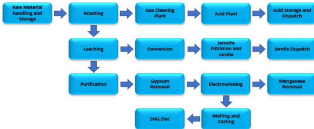
Figure 3: Gamsberg Smelter Process Flow 4
