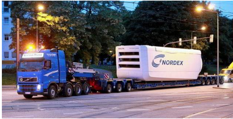
Figure 7-2 Example of Nacelle Transport ( Recharge News )
