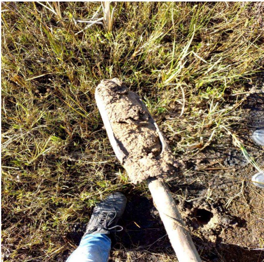
Figure 5-7 - Soil Sample taken at 50-60 cm in the seasonal zone of the wetland
