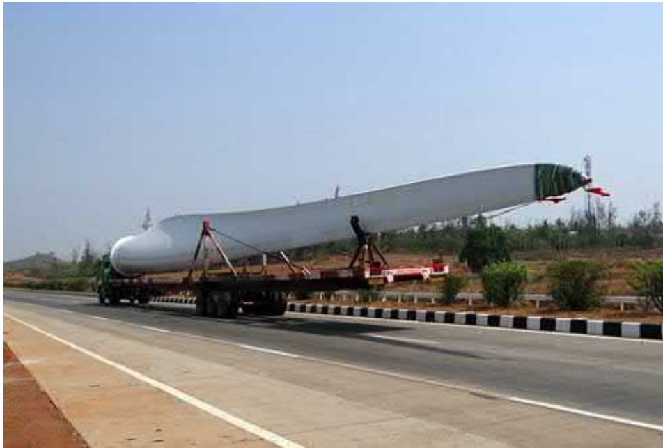
Figure 4-2: Blade transport (Froese, 2019)
