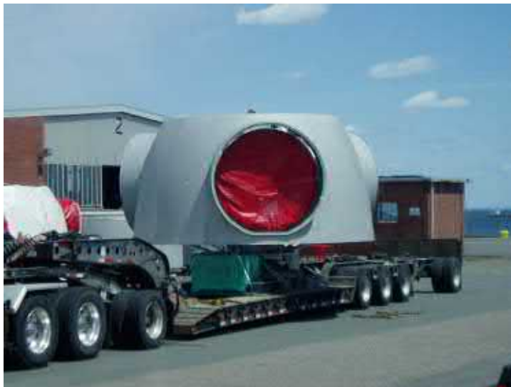
Figure 4-4:Transporting the rotor hub (Richardstransport, n.d.)
