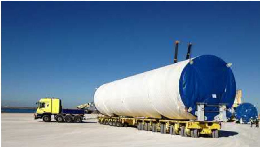
Figure 4-3:Transporting the Tower Sections (Montiea, 2014)
