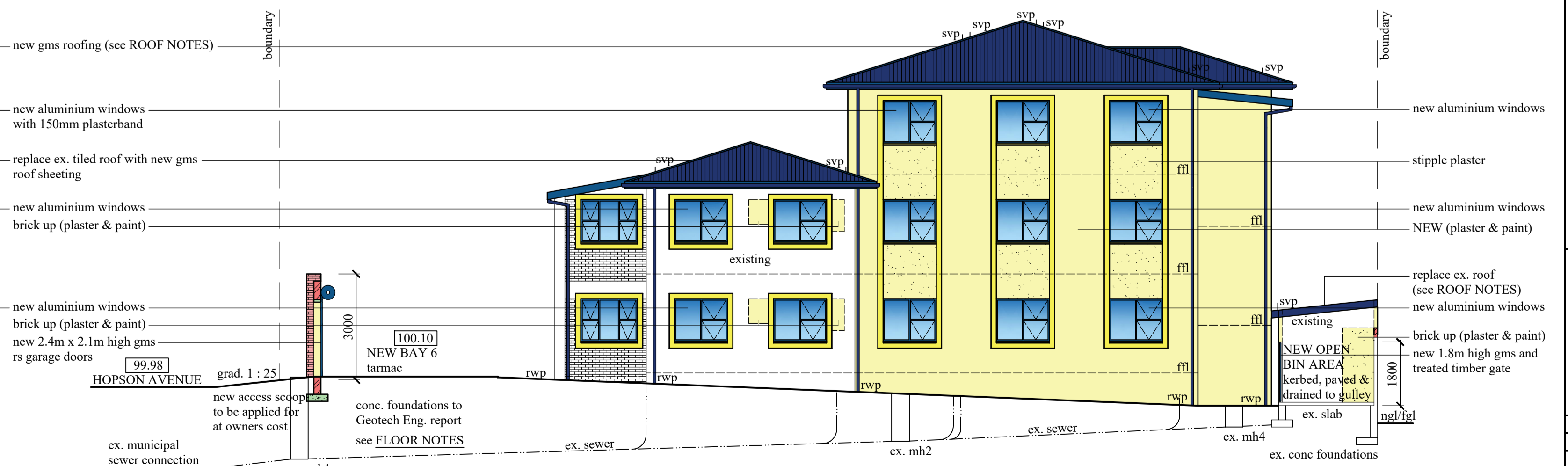
SOUTH WEST ELEVATION / SECTION D - D connect all new plumbing to ex. sewer
