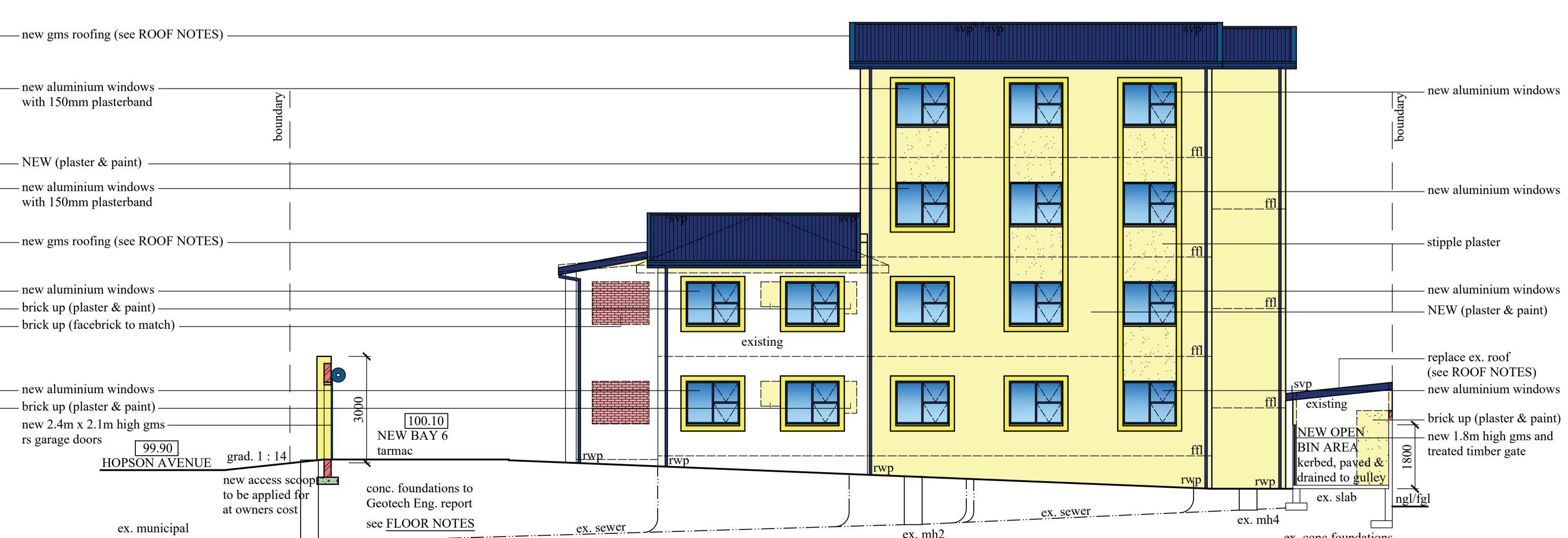
SOUTH WEST ELEVATION / SECTION D - D connect all new plumbing to ex. sewer
