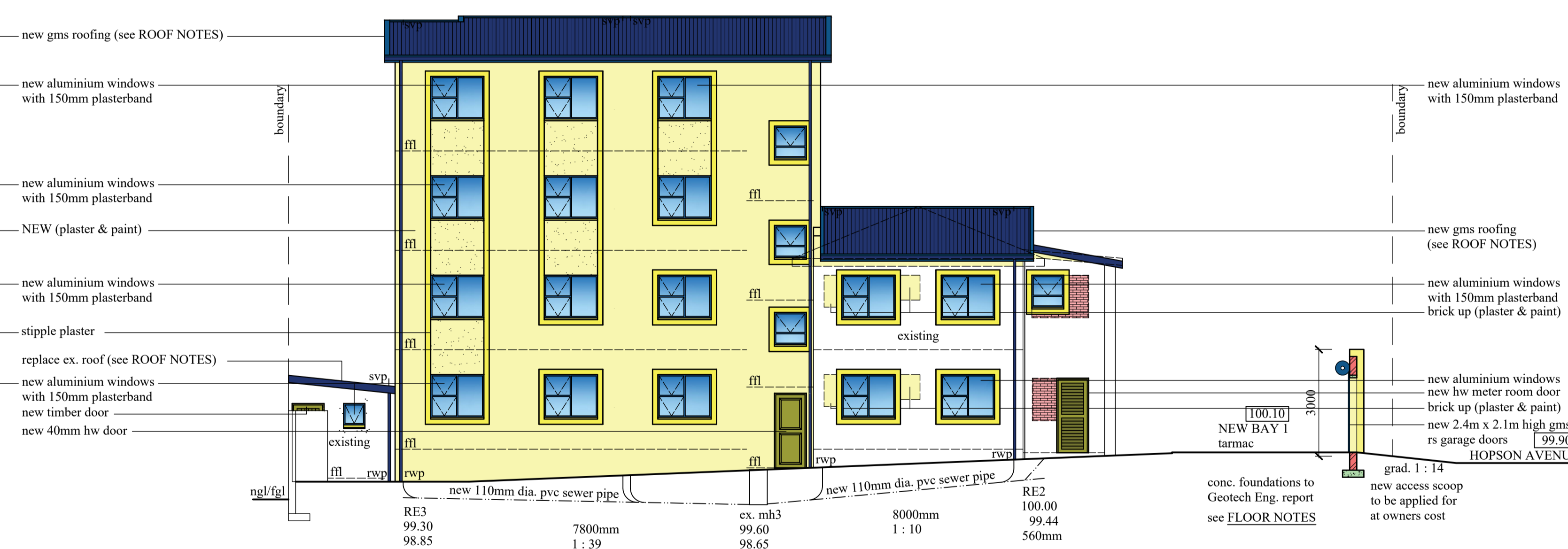
NORTH EAST ELEVATION / SECTION C - C connect all new plumbing to ex. sewer
