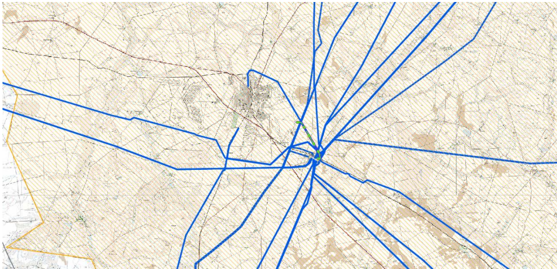
Figure 2: Grid connection corridor (green) in relation to existing electricity transmission infrastructure (blue) converging on the Hydra Main Transmission Substation near De Aar, with a small portion of the large ESA and IBA covering a large portion of the region indicated with orange hatching.
