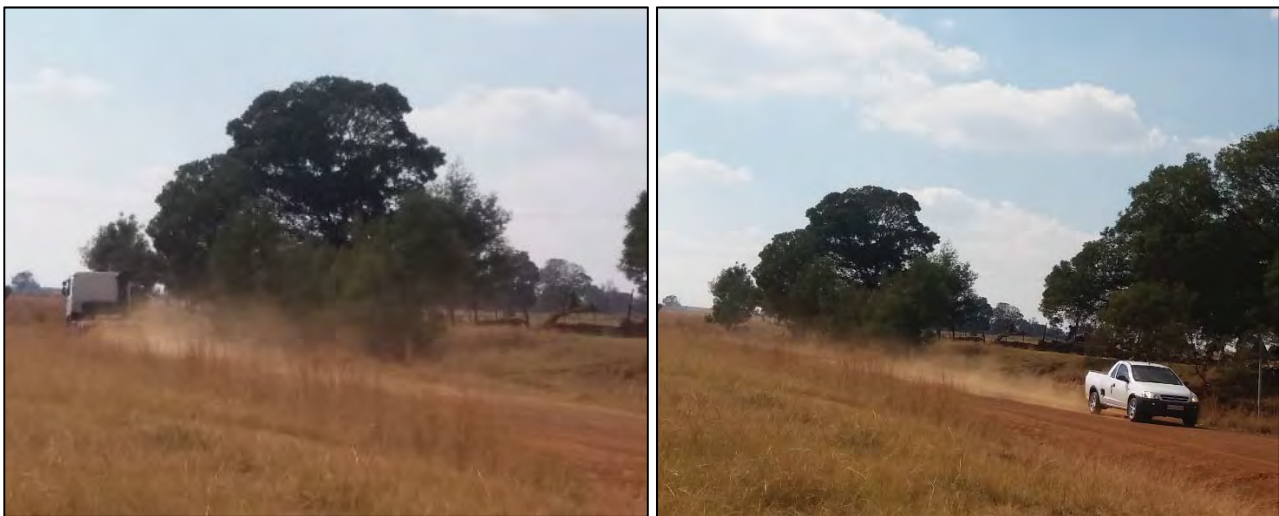
Figure 23: Dust generated on D648 by heavy (left) and light (right) motor vehicles (Golder, 2016)
