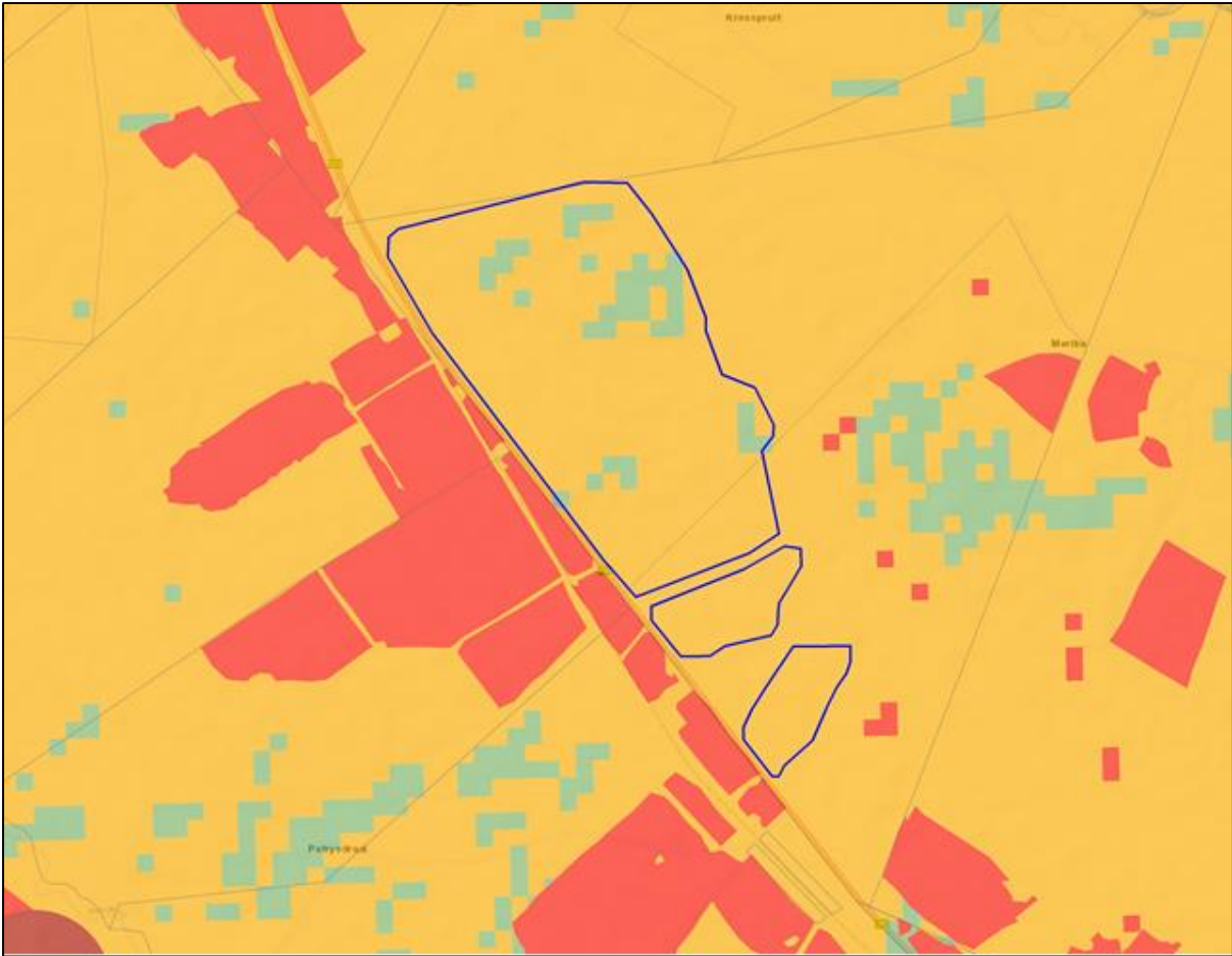
Figure 25: Proposed development footprint overlaid on agricultural sensitivity (green=low sensitivity; yellow = medium, red = high)
