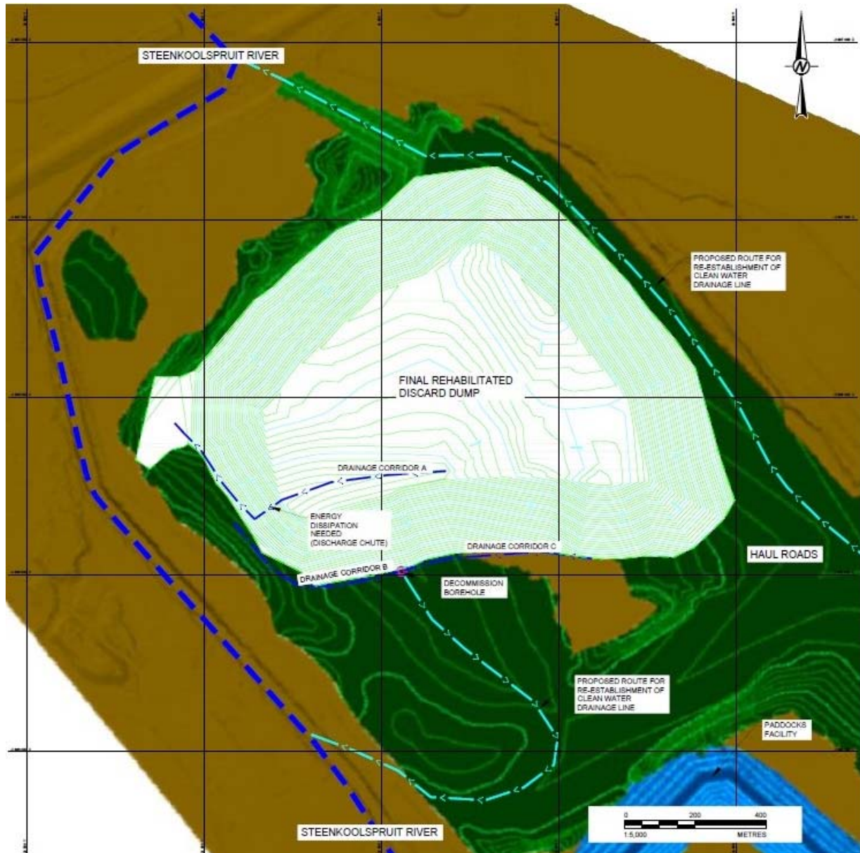
Figure 18: Final closure layout and drainage – South Pit Course Discard Dump (Golder Associates (Pty) Ltd (c), April 2018)
