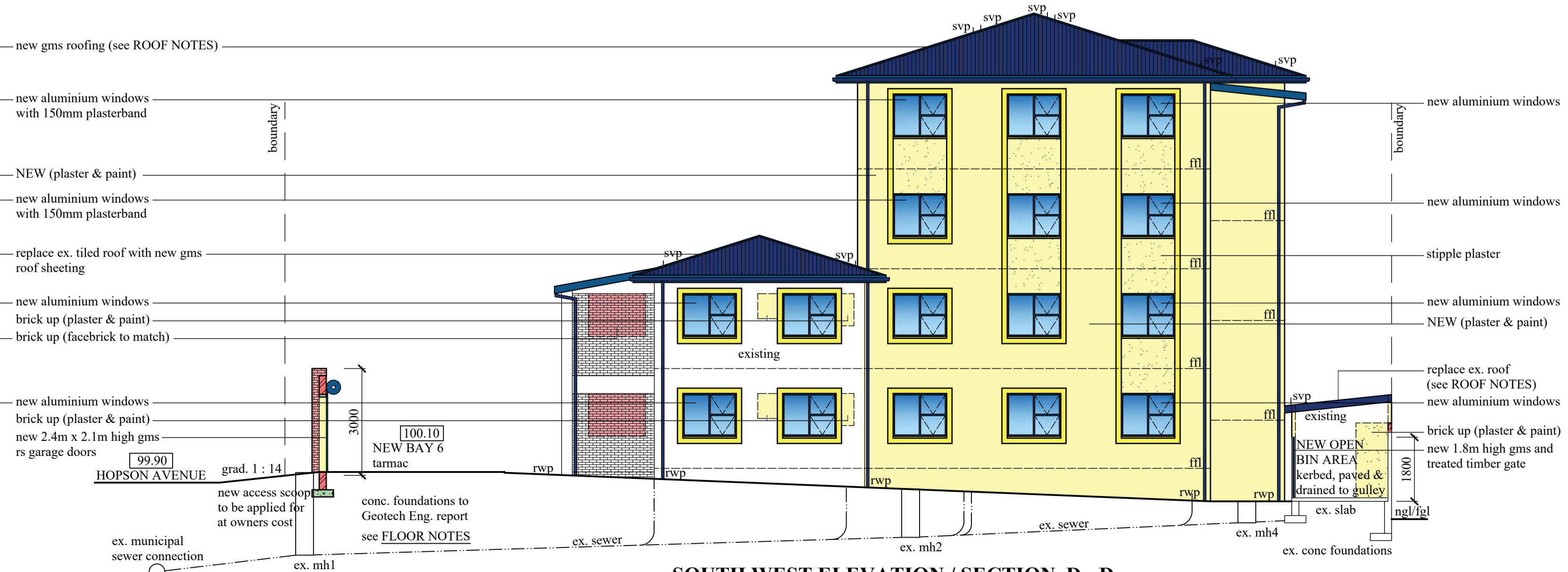
SOUTH WEST ELEVATION / SECTION D - D connect all new plumbing to ex. sewer
