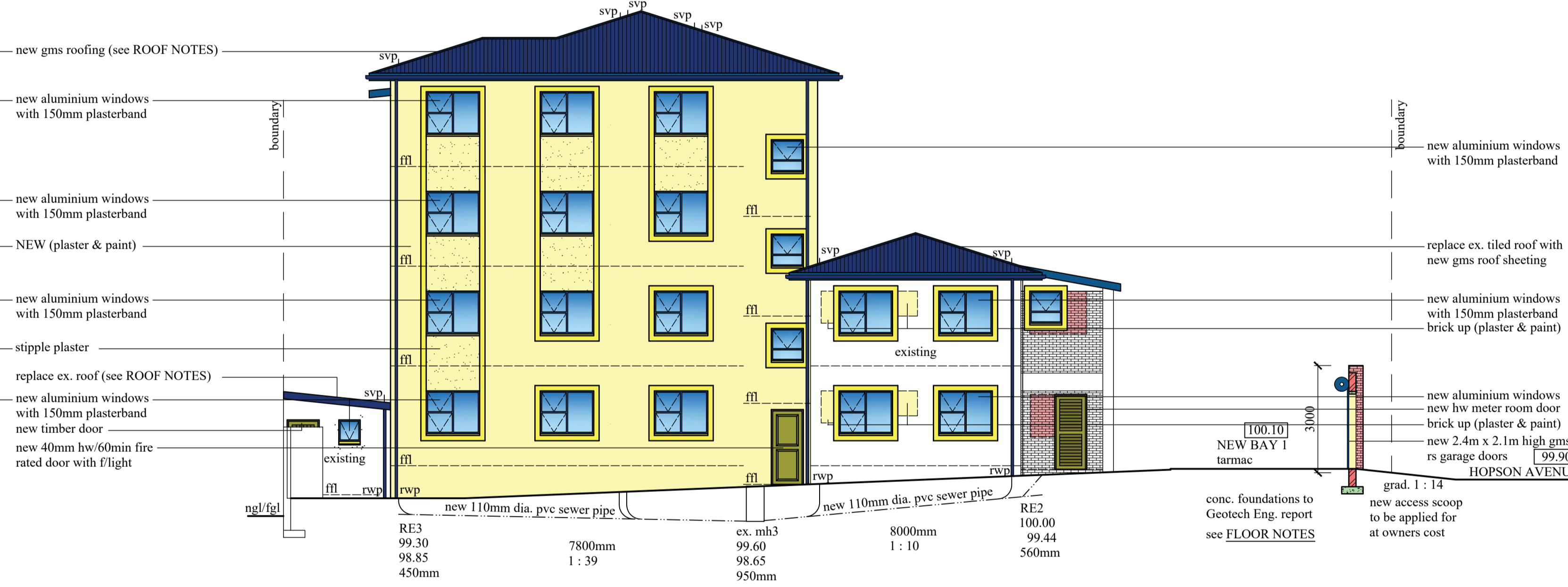
NORTH EAST ELEVATION / SECTION C - C connect all new plumbing to ex. sewer
